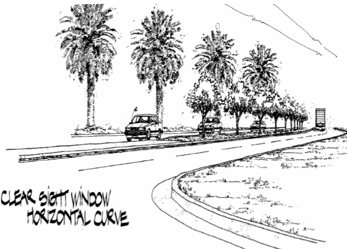
Source: Florida Highway Landscape Guide - 1995 SIGHT DISTANCE AS IT RELATES TO MEDIANS AND MEDIAN OPENING DESIGN
