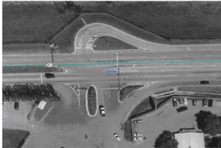
Jug-handle at a Miami horse race track specifically designed for horse trailers
