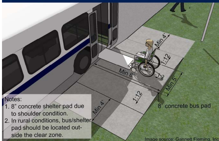
Figure 3.4: Bus Pad in Rural/Suburban Conditions
