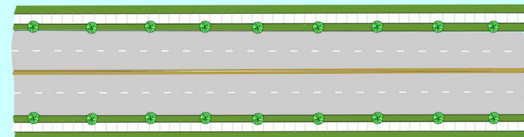
PROJECT SEGMENT - WIDENING FROM 2 LANES TO 4 LANES
