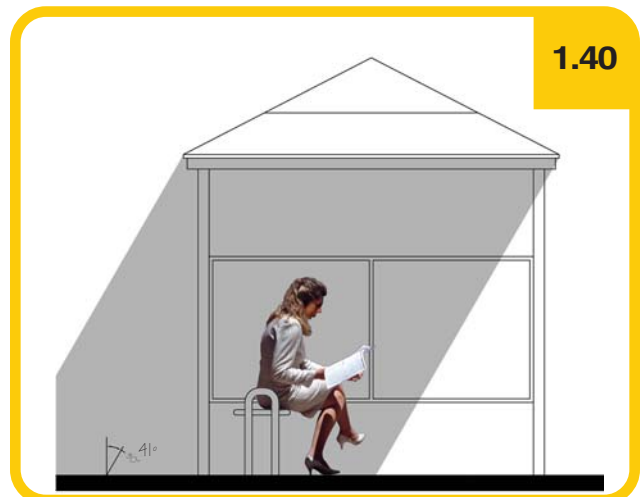
Approximate angle (41°) of the sun during late afternoon peak commuting hours in mid-summer in central Florida for a southwest facing bus shelter.
