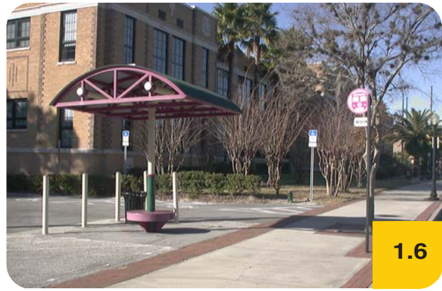
A bus stop sign placed between the sidewalk and the travel lane near a sheltered bus stop.
