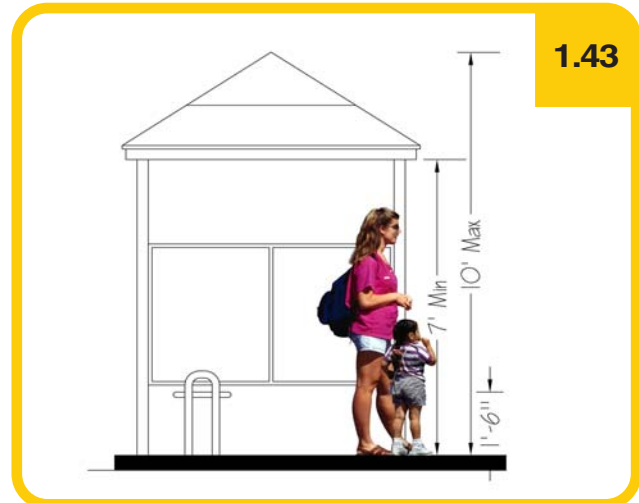
Cross section of a mid-size shelter with typical vertical dimensions.
