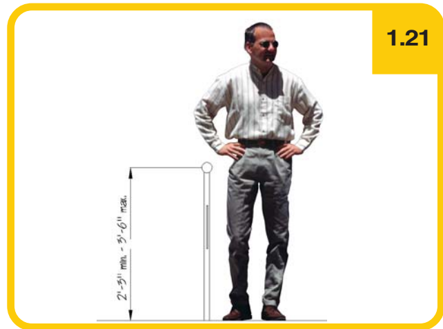
Correct height dimensions for bus stop leaning rails.
