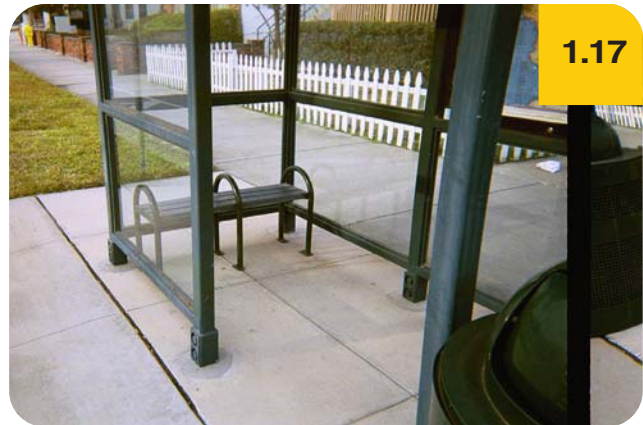
Bus bench within a bus shelter that allows sitting patrons a clear view of on-coming buses.
