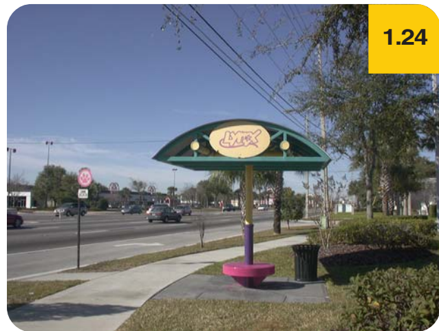
Correct location of a trash receptacle at a bus stop in Orange County, FL.
