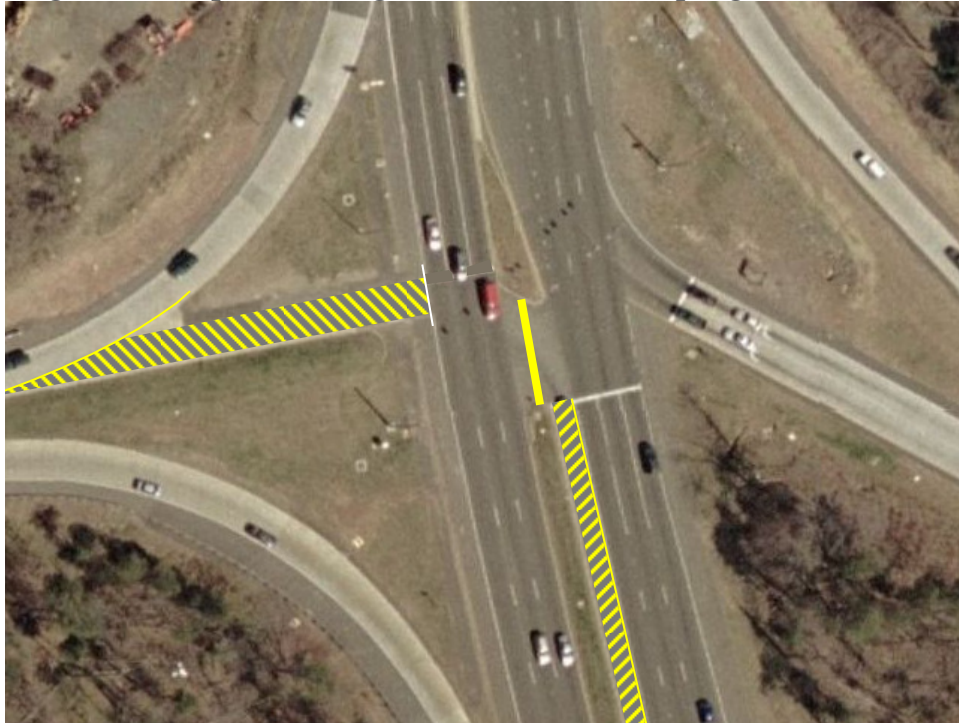
Figure 5: Proposed Changes to I-66 North Ramp Signal at Route 28
