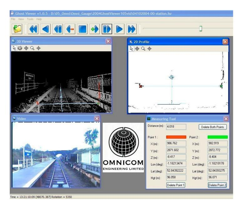
It also enables track clearances to be dynamically viewed and measured in the software within both the point cloud and the video imagery.
