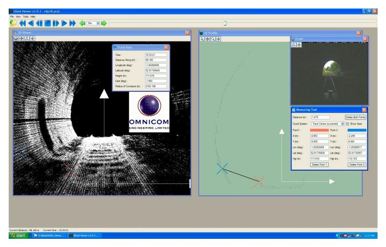
The image on the left represents the point cloud. The image on the right represents a slice from the point cloud which can be used to determine the tunnel geometry. Each view has a virtual camera capability with the three-dimensional view enabled for rotation, zoom, pan and tilt allowing close-up inspections of interest within the tunnel. Note the refuge on the left, and piping on the right.
