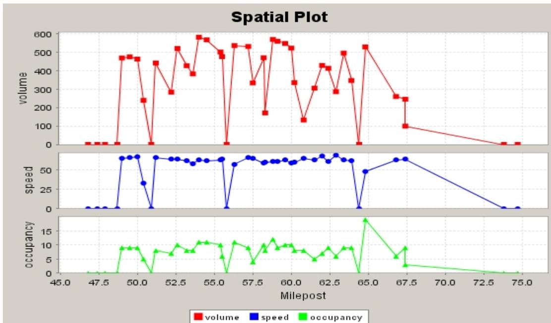
**Figure 3.** Shows speed, volume, and occupancy of I-66 Eastbound on 10/16/2006.
