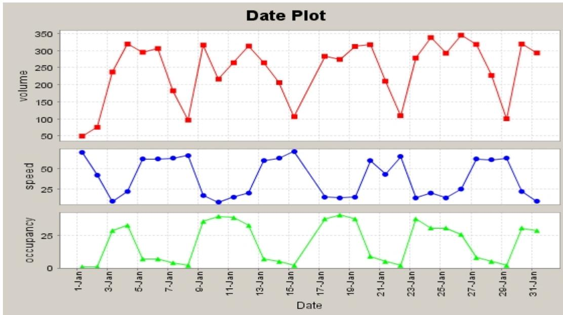
**Figure 2.** Shows speed, volume, and occupancy of station 271 from 1/1/2006 – 1/31/2006.
