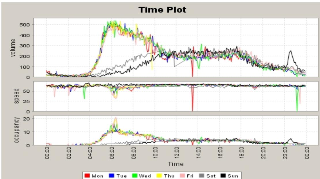
Figure 6. Shows speed, volume, and occupancy of all days in the week for station 121 for 2/1/2006-2/7/2006.
