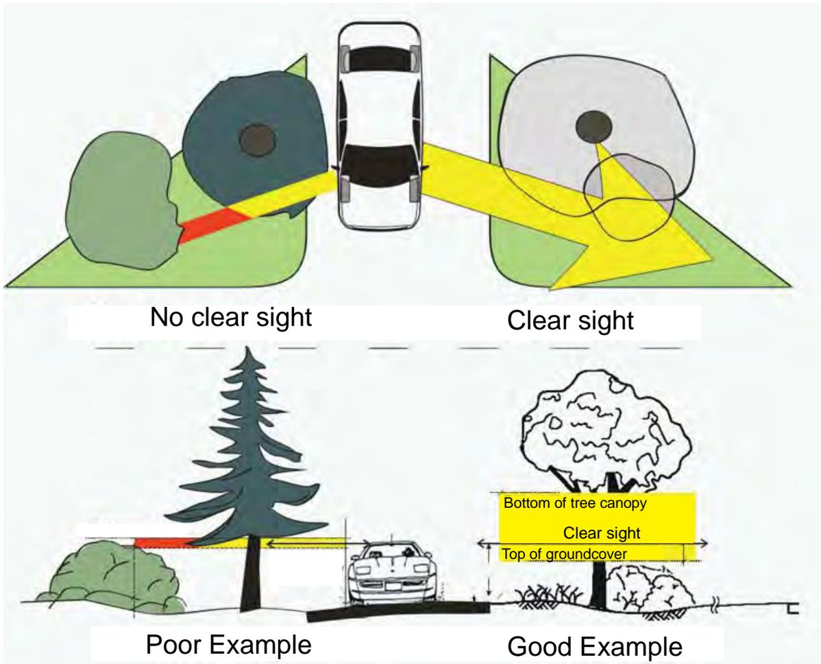
*The intent of this standard is to provide a window with vertical limits of not less than 5' above and 18" below the sight line datum, and horizontal limits defined by the limits of clear sight.*
