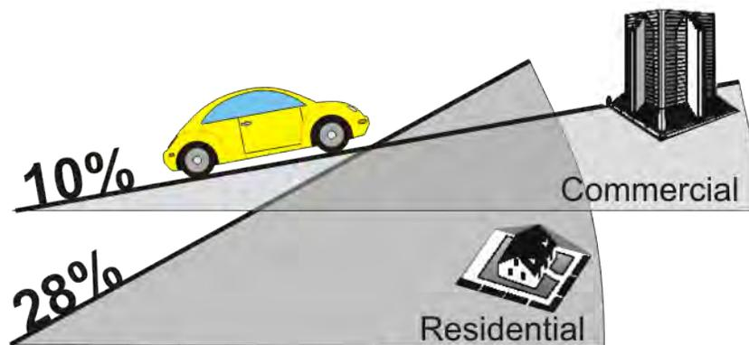
While these may be the maximum practical grades, it is much better to use smaller grades. **Research has shown that grades less than 14% for low volume driveways and grades less than 5% for higher volume driveways are more desirable.**
