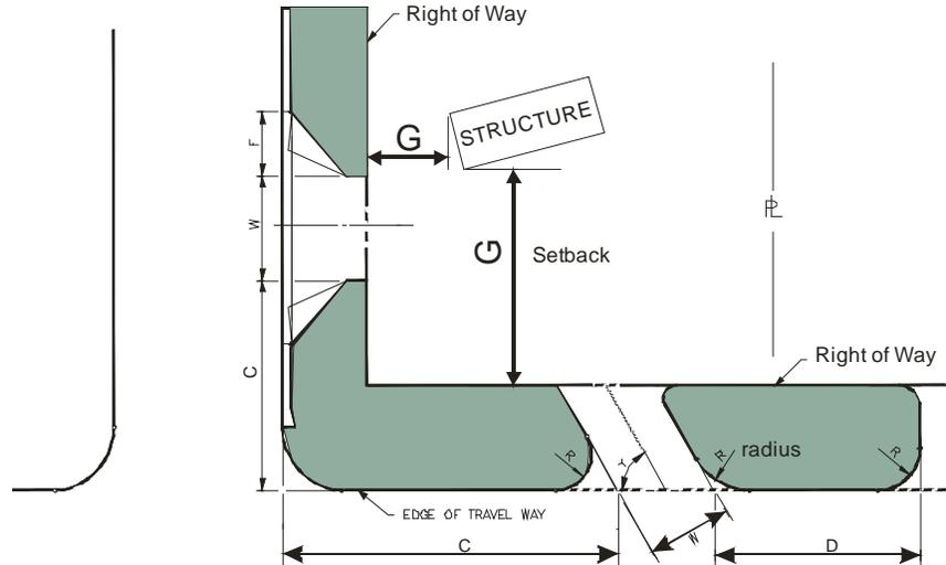
**G = 12 feet or greater, however it needs to be placed so “all vehicular queuing, stacking, maneuvering, standing, and parking to be carried out completely beyond the right of way line”**
