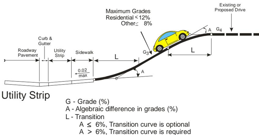
Guidance for Driveway Design in the Design Standards and in the Plans Preparation Manual (Curb and Gutter Sections)
