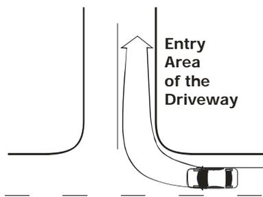
The entry area is probably the most critical portion of driveway width. The entry width should be sufficient to allow a vehicle to:
