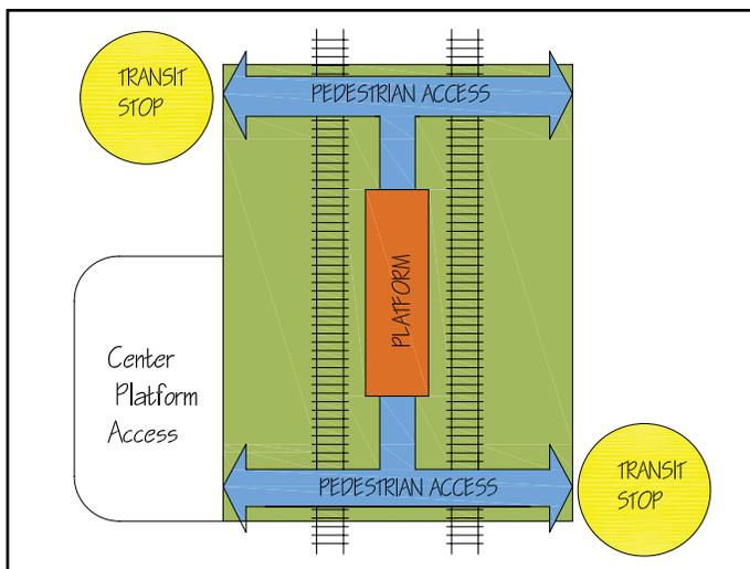
**Figure 3.27** | Diagram of a central platform station.
