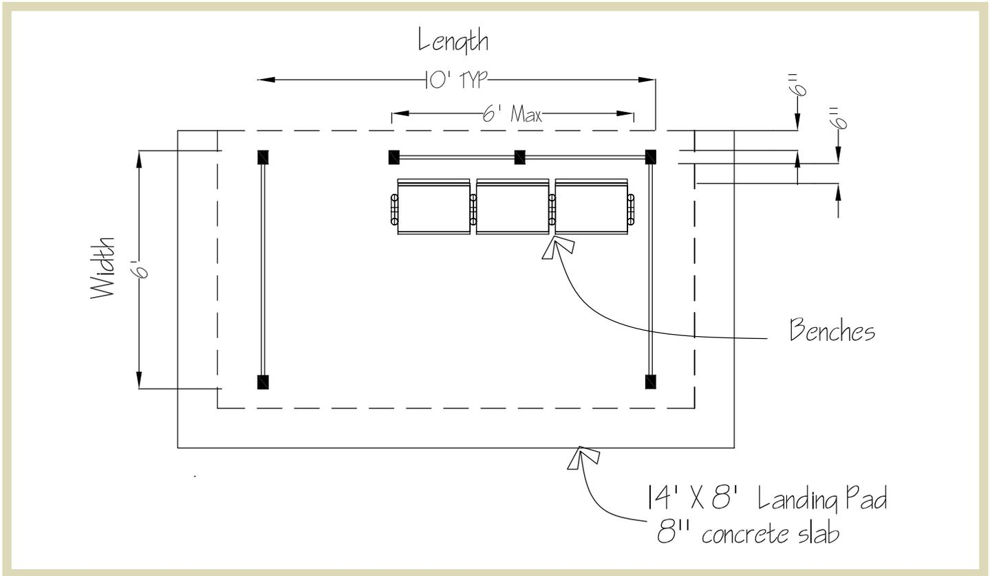
**Fig 1.28** | Typical dimensions of a mid-sized bus shelter.
