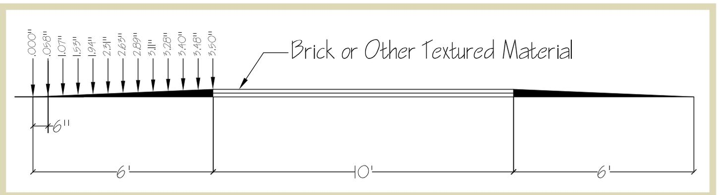
Figure 2.26 | A raised pedestrian crosswalk in cross section.
