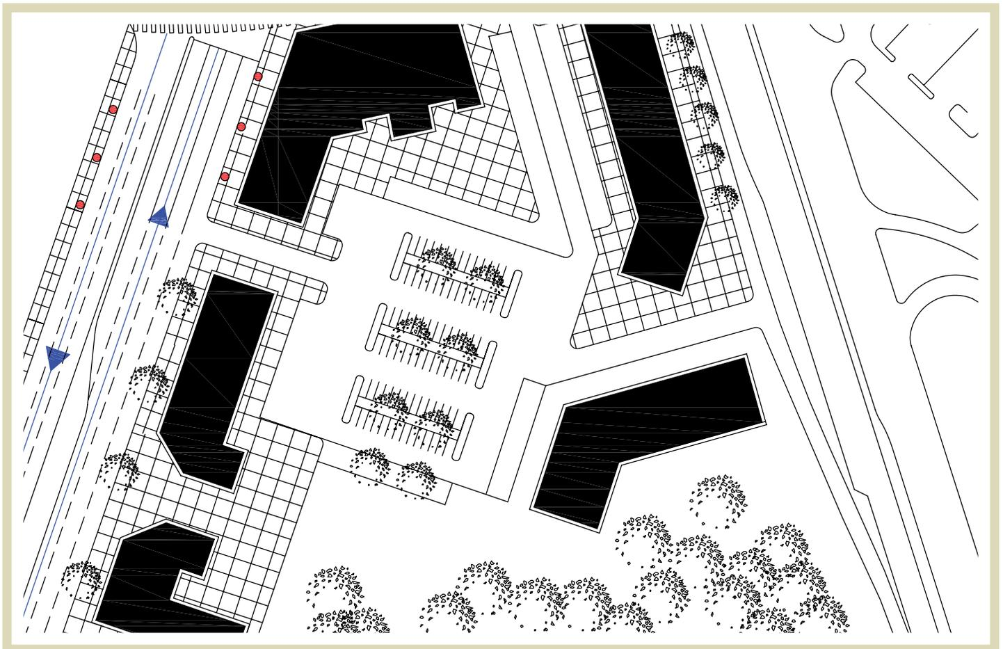
**Figure 4.10** | Shopping centers can be made more accessible to transit riders and pedestrians by locating parking at the center and providing primary transit stops along high-traffic corridors.
