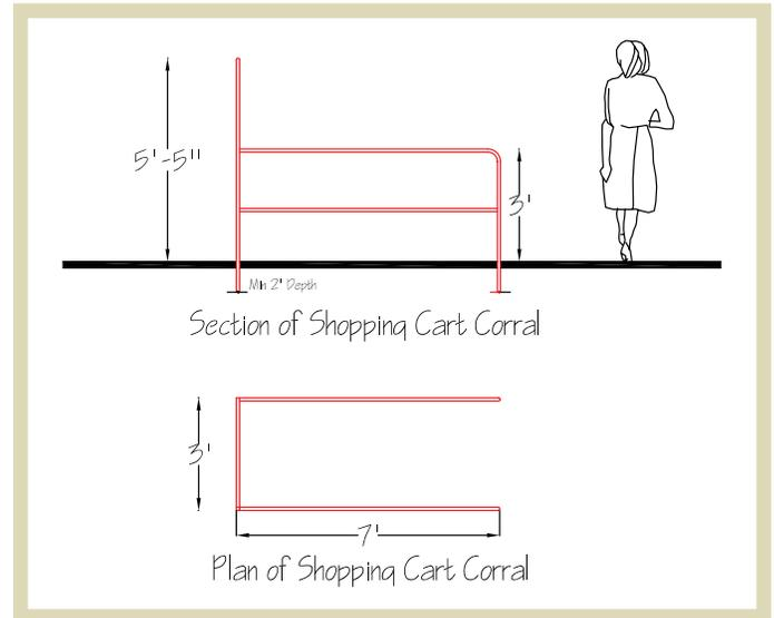
**Fig 1.65** | Typical vertical and horizontal dimensions for shopping cart corrals.
