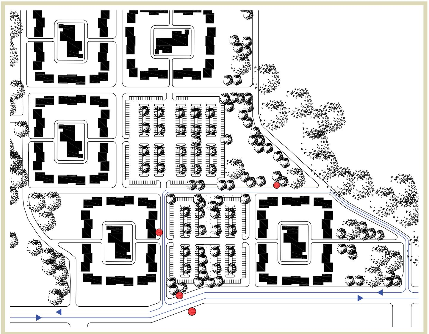
**Figure 4.6** | Transit friendly multi-family residential units. Bus stops are indicated in red dots in plan.
