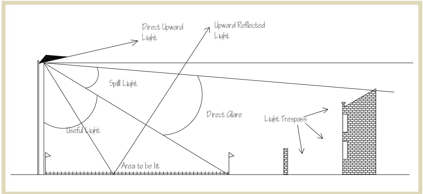
**Fig 1.44** | Light pollution is wasteful of energy resources and causes dangerous glare to spread into the right of way.
