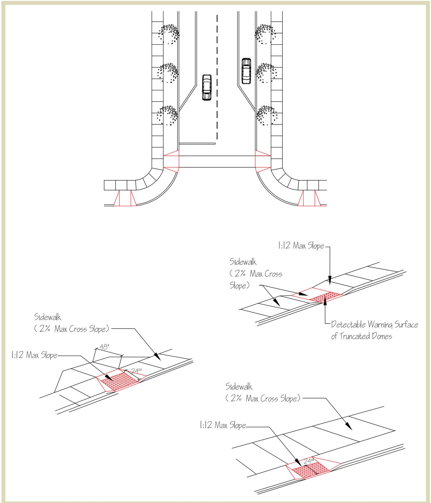
**Figure 2.23** | Alternatives for accessible curb ramps.
