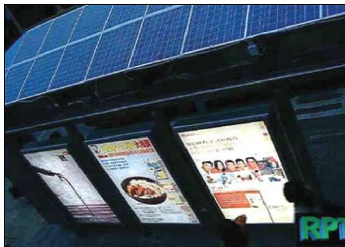
**Fig 1.36** | The solar powered bus shelter illuminates its information systems and advertising panels with power generated by photovoltaic panels, independent of the electricity grid.
