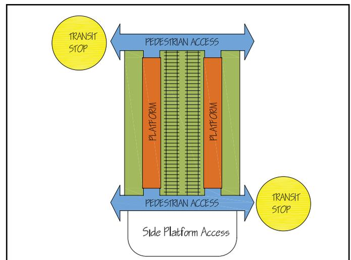
**Figure 3.28** | Diagram of a side platform station.
