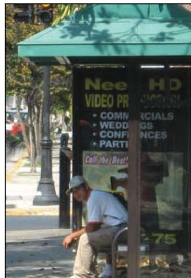
**Figure 1.10** | Bus bench within a bus shelter that allows sitting patrons a clear view of oncoming buses.
