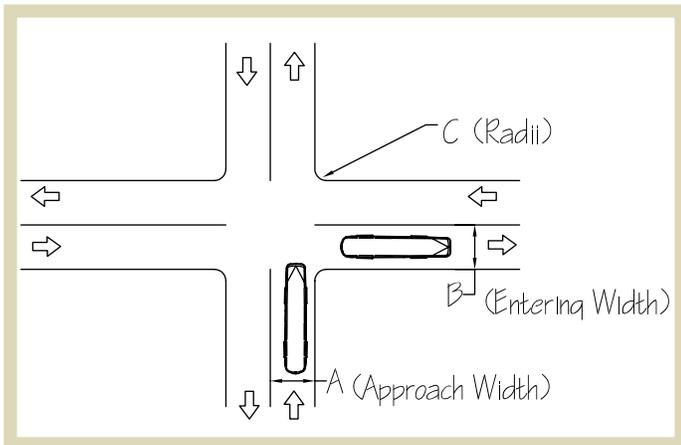
**Figure 2.13** | Important measurements related to bus turning movements.
