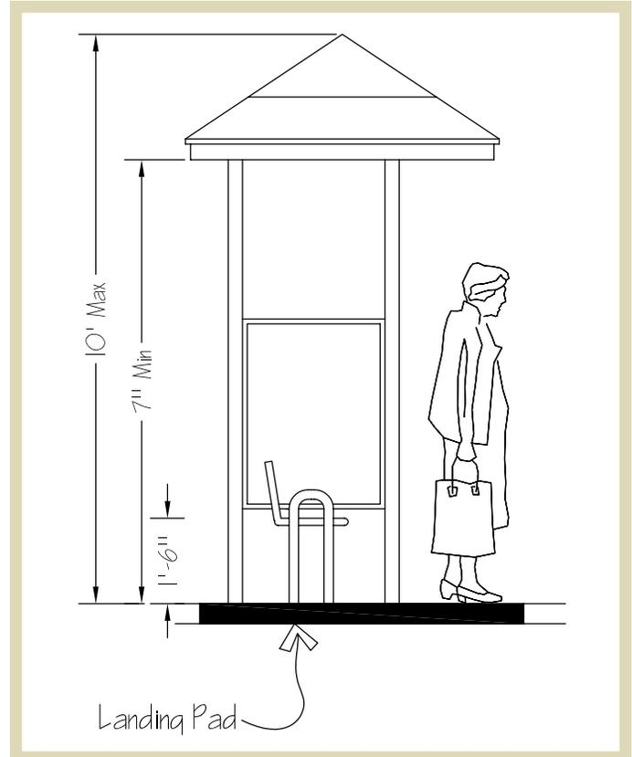
**Fig 1.26** | Cross section of a small shelter with seating with typical vertical dimensions.
