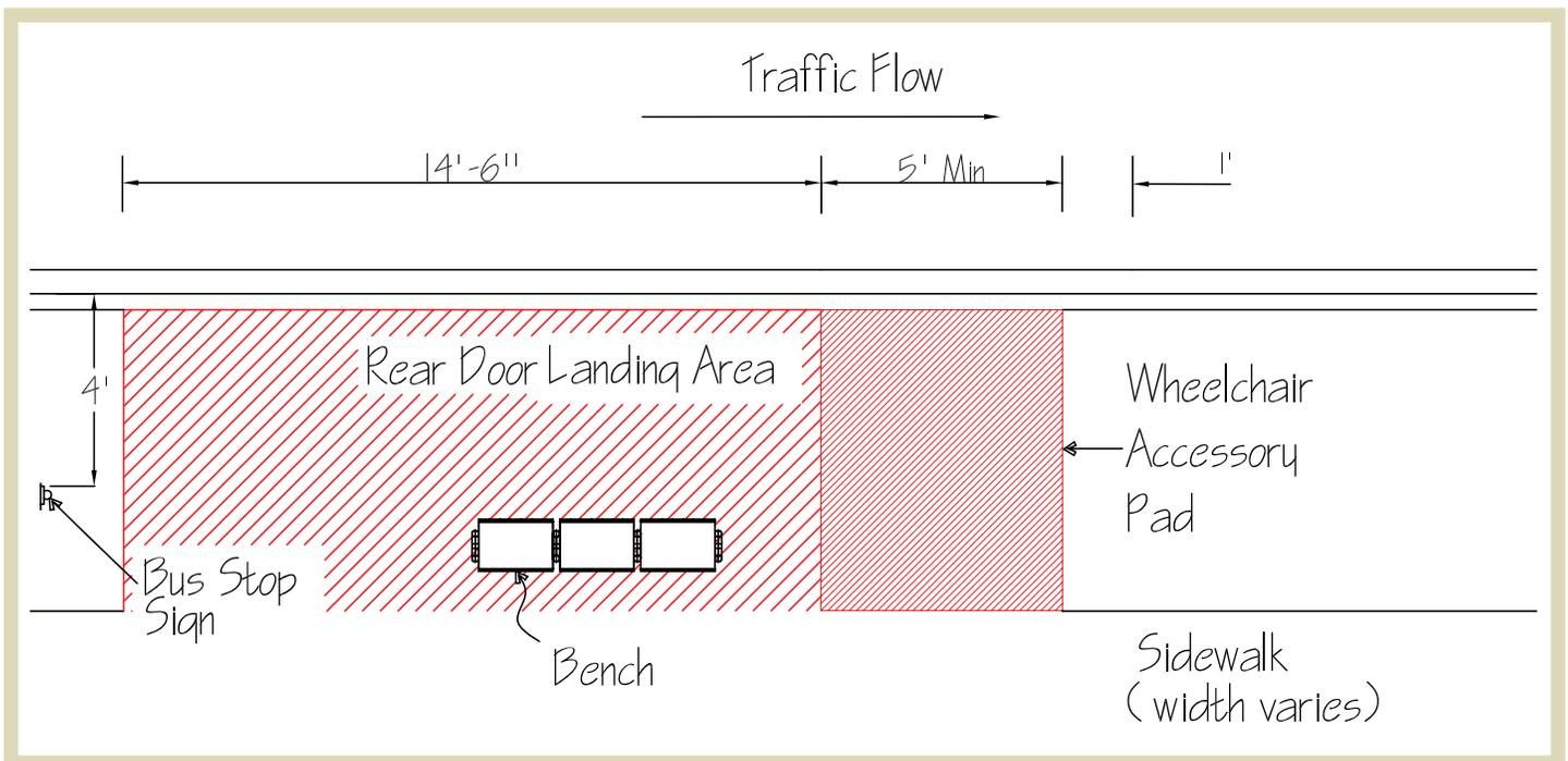
**Figure 1.17** | Bus stop pad without shelter but with bench.
