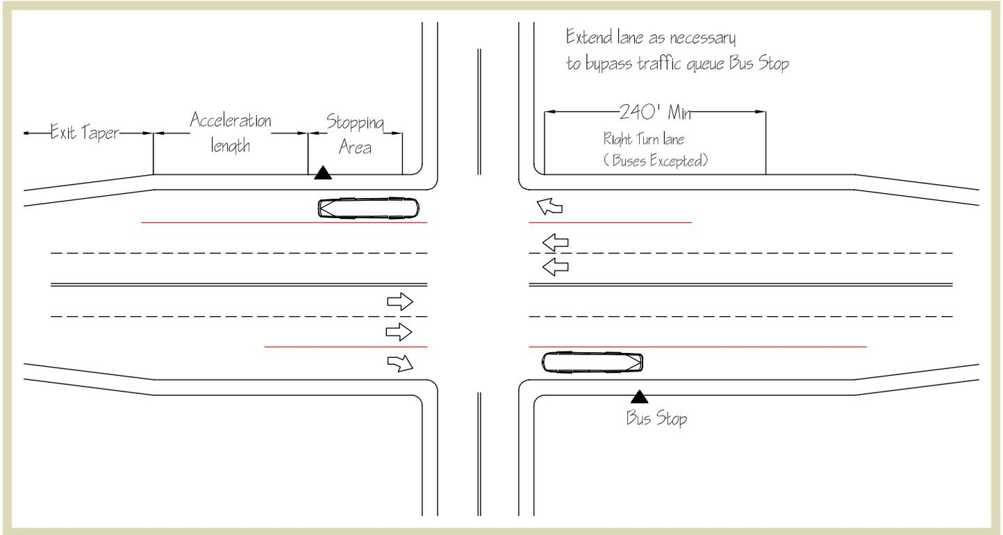
**Figure 2.18** | Typical configuration and dimensions for a queue jumper bus bay.
