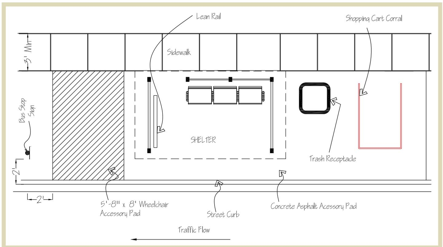
**Fig 1.64** | Appropriate location of a shopping cart corral at a sheltered bus stop.
