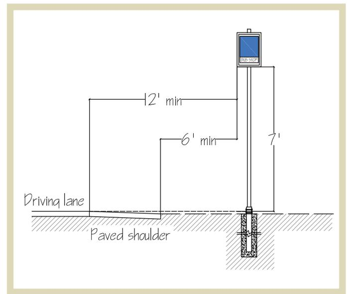
**Figure 1.6** | Dimensions for a bus stop sign placed adjacent to the travel lane of a road without curb and gutter.
