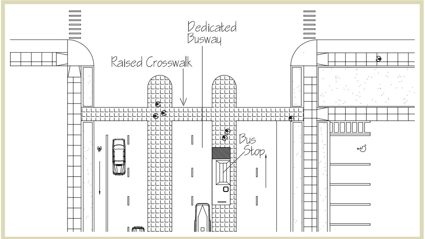
**Figure 3.10** | Detailed transit mall plan.
