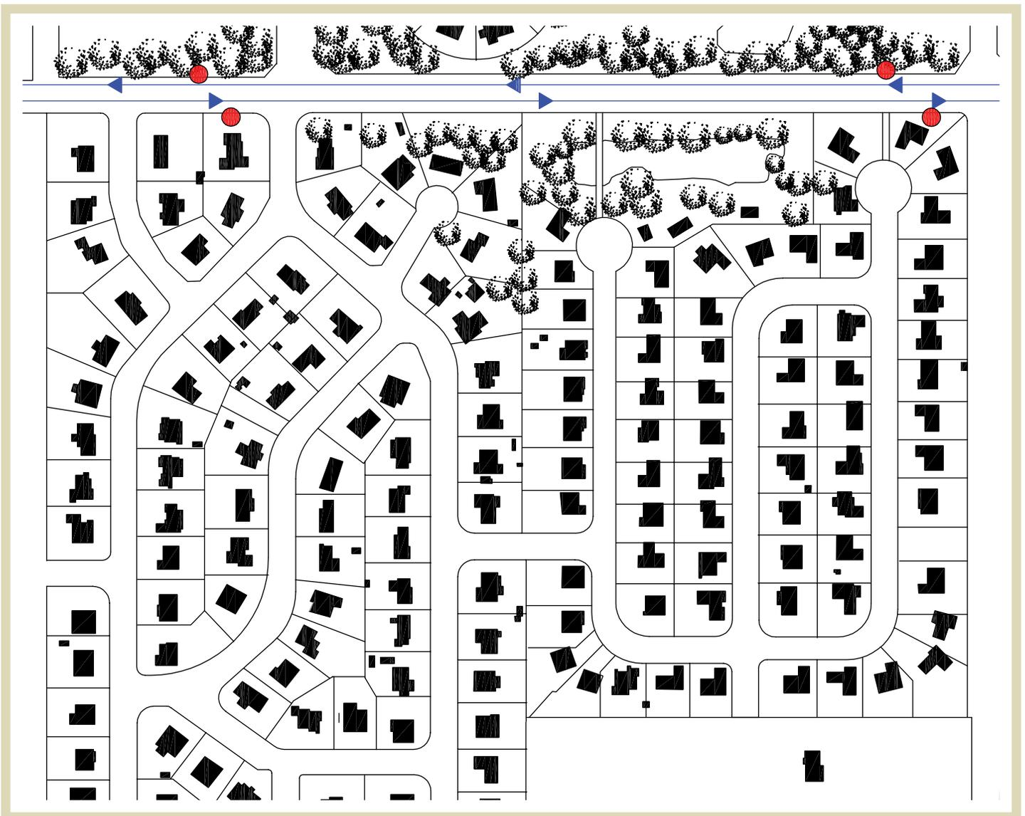
**Figure 4.3** | Traditional single family residential development with cul-de-sacs. Bus stops are indicated in red dots in plan. Bus stop locations are indicated by red dots and bus routes are shown in blue.
