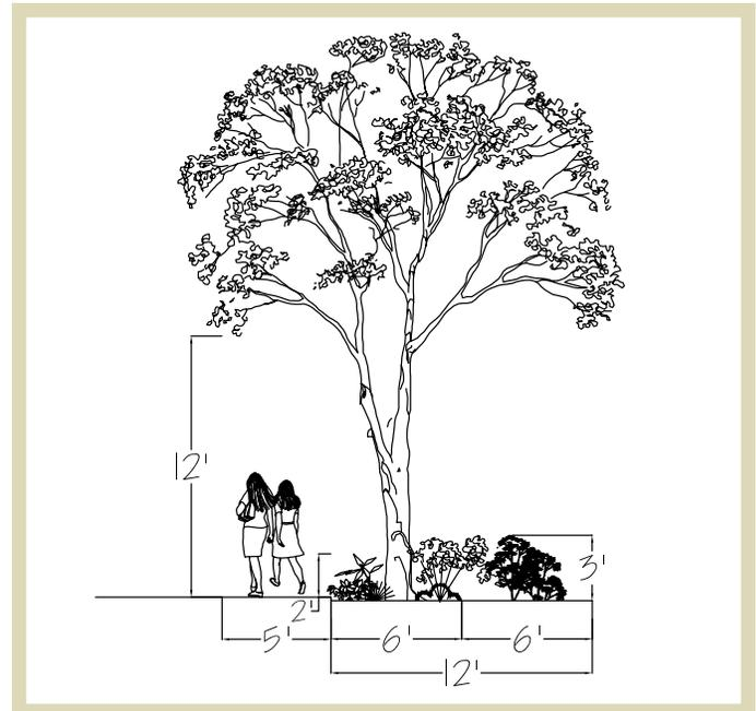
**Fig 1.47** | Appropriate locations and vertical dimensions for landscaping adjacent to a sidewalk.
