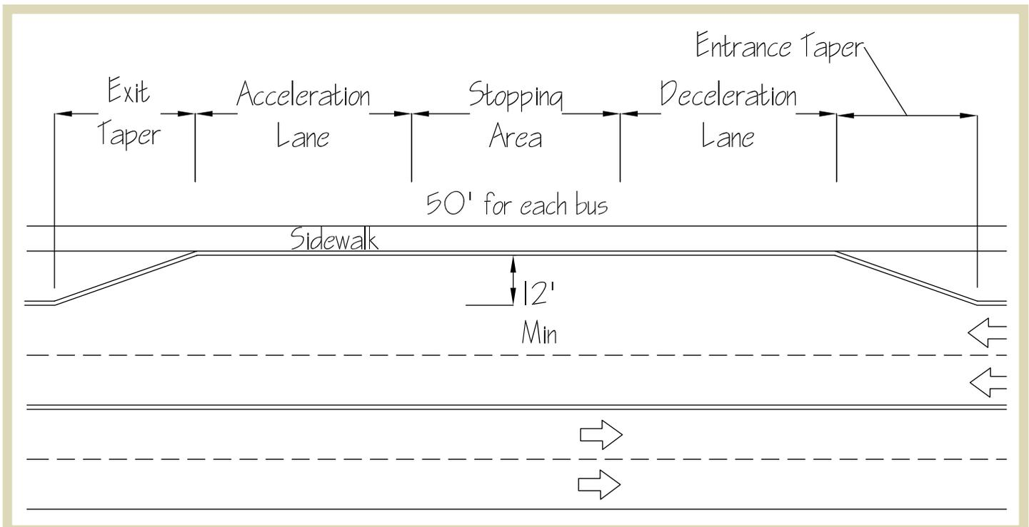
**Figure 2.17** | Critical dimensions related to bus bays.
