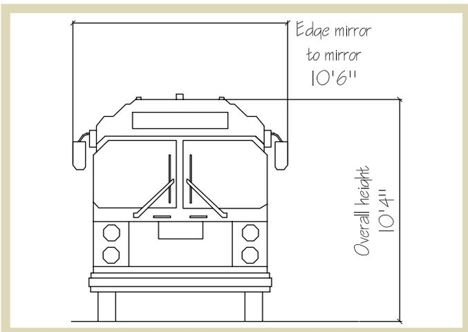
**Fig 2.8** | Front view of an articulated bus.
