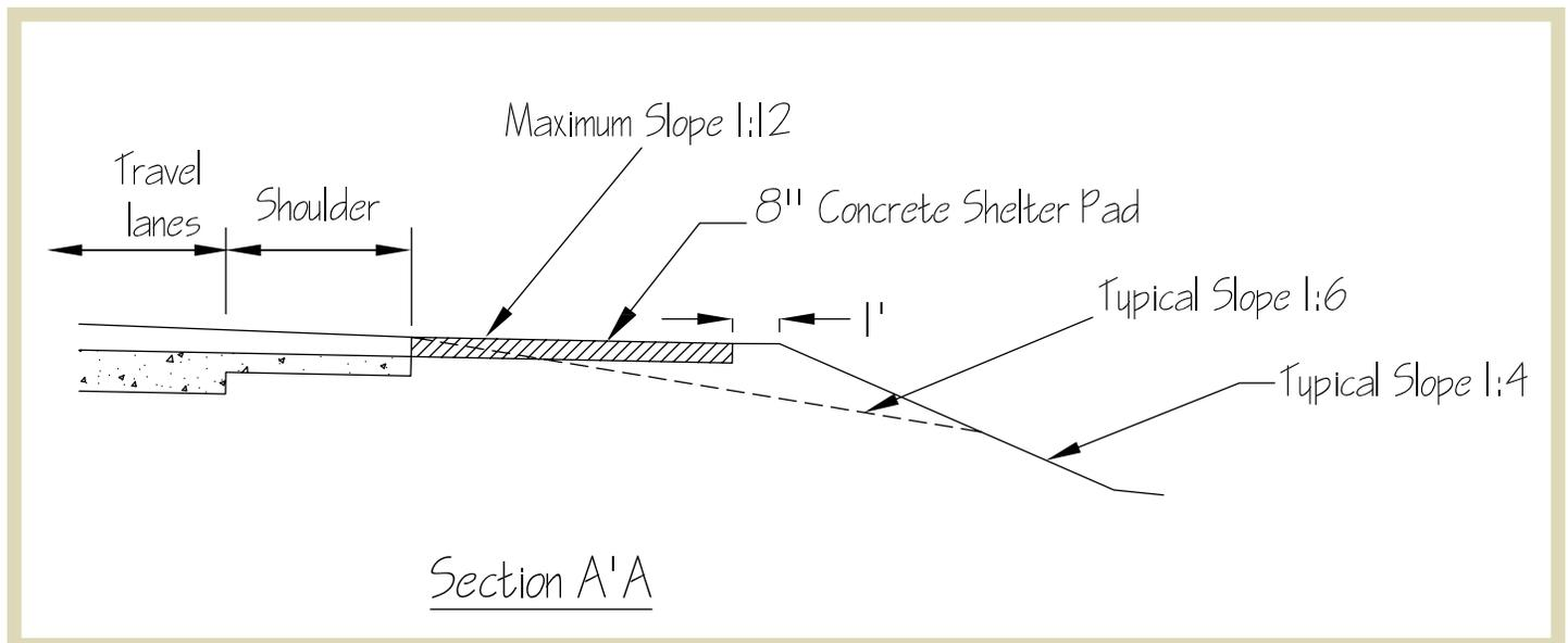
**Figure 1.20 b** | Cross-section showing landing pad configuration for rural bus stop.
