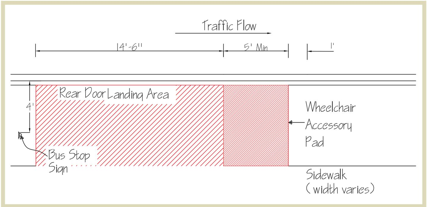
**Figure 1.18** | Bus stop pad without shelter and bench.
