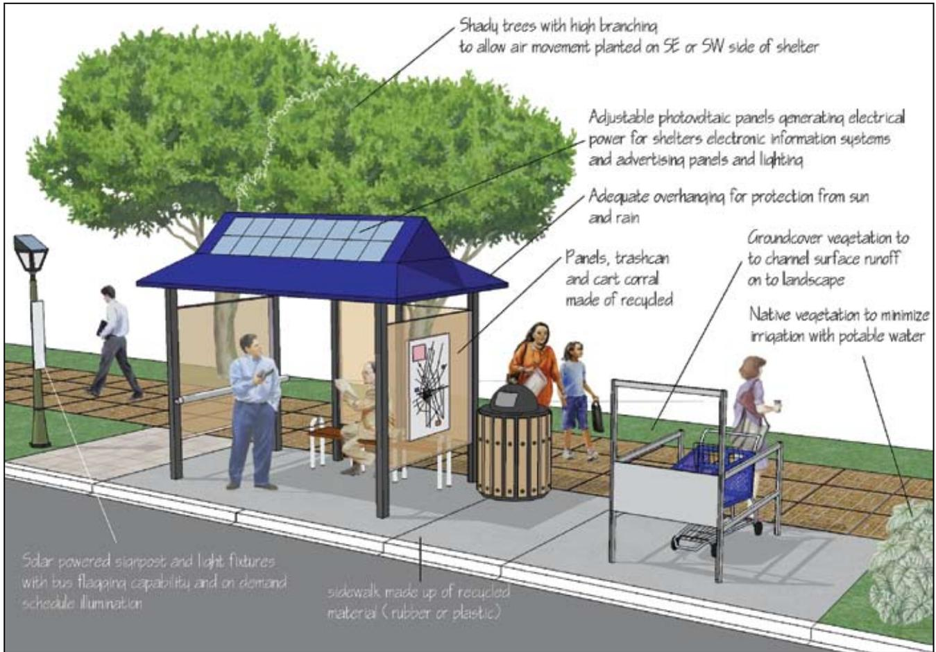
**Fig 1.35** | A bus stop designed according to “green building” design principles.
