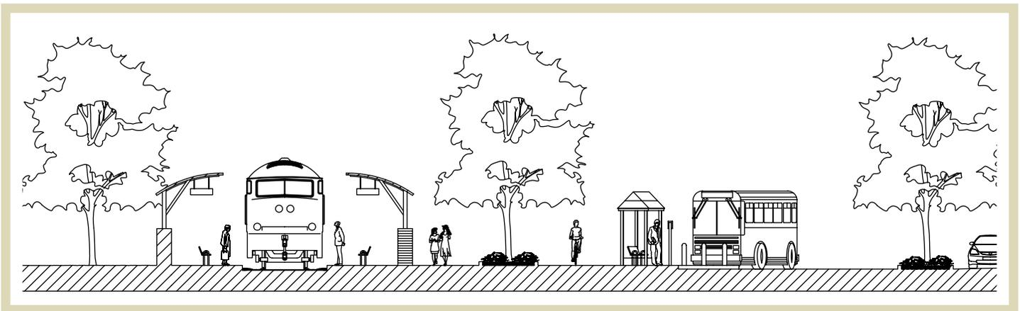
**Figure 3.26** | Section showing at-grade tracks and single platform connecting both modes of transit.
