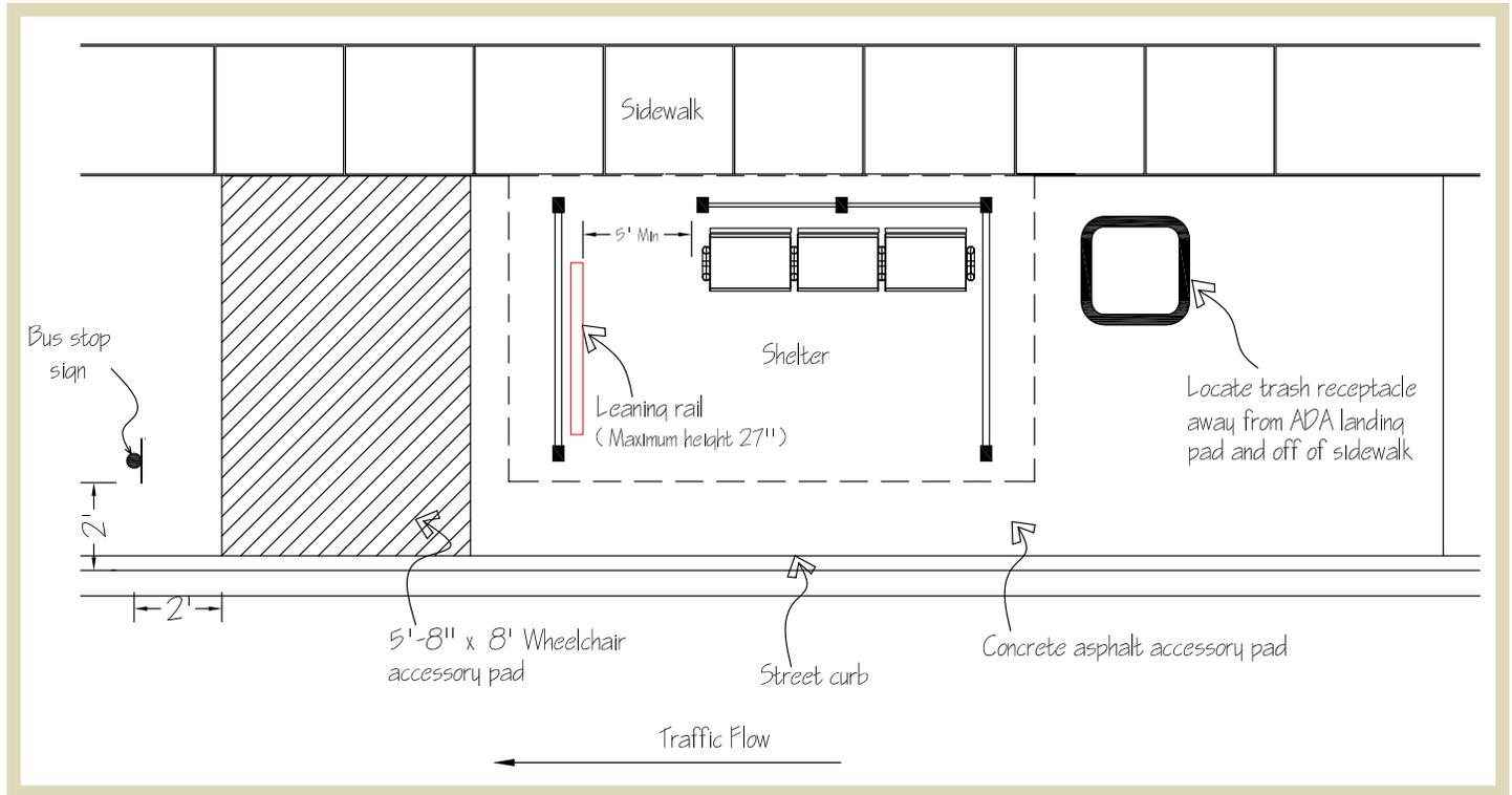
**Fig 1.50** | Correct location of a leaning rail located inside a bus stop shelter.
