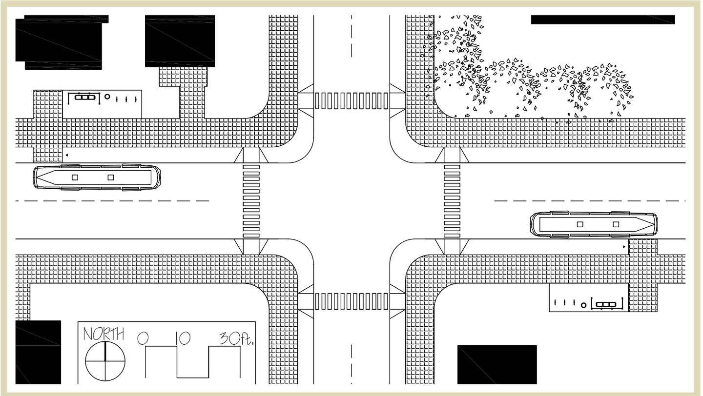
**Figure 3.1** | Typical curb-side, on-line sheltered bus stops located at the far-side of an intersection.
