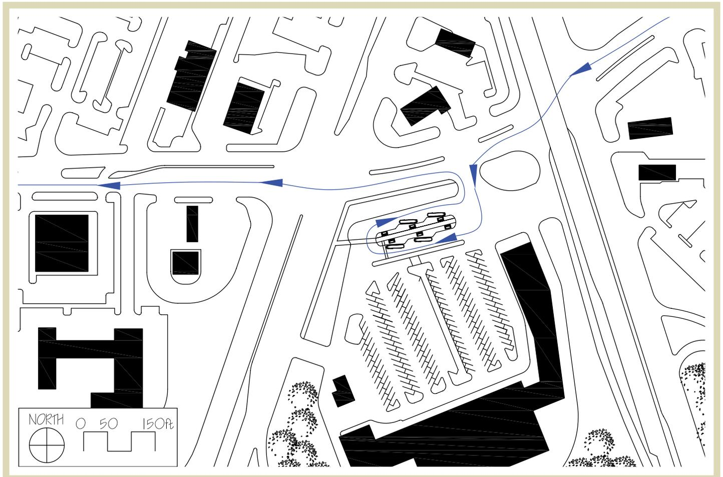
**Figure 3.13** | A transit center located within a retail center near a highway interchange.
