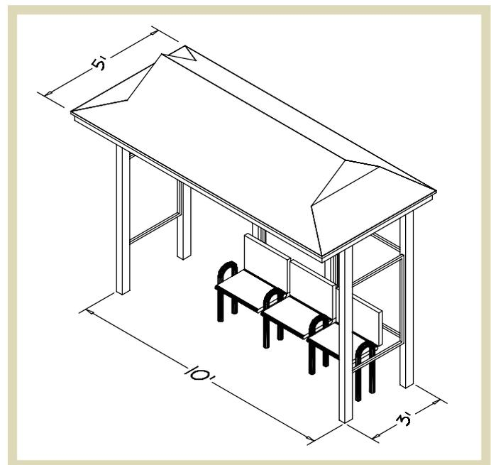
**Fig 1.27** | Bus shelter with seating shown in three dimensions. Plan view of the same small bus shelter with a leaning rail shown in Figure 1.25.
