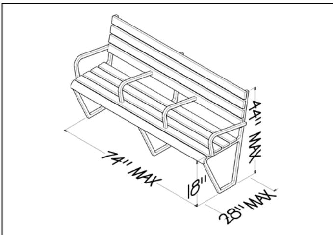
**Figure 1.14** | The required dimensions for divided bus benches with backs.
