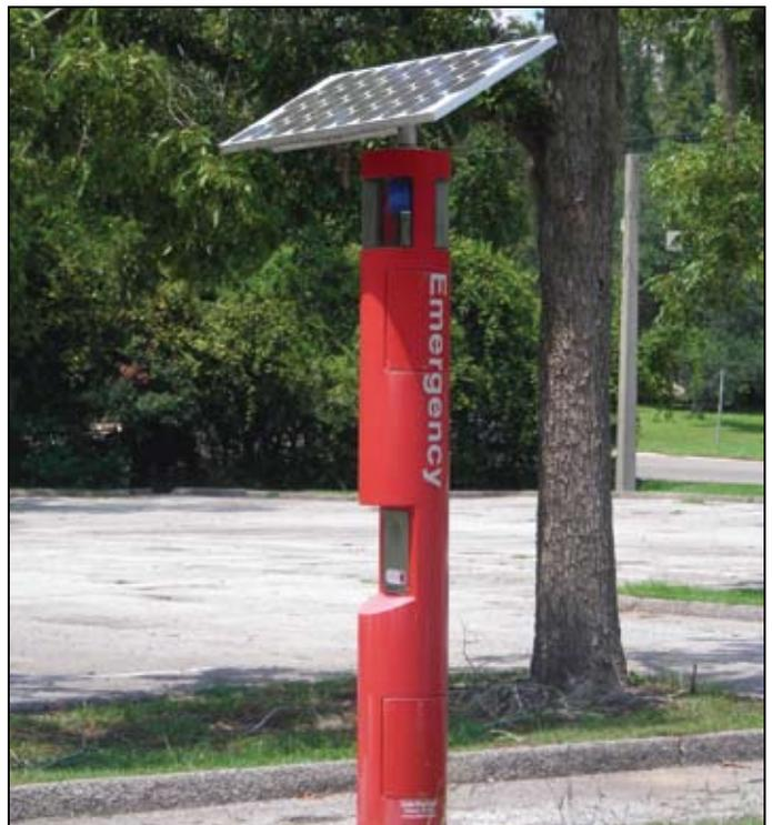
**Fig 1.67** | A typical solar powered emergency call box.
