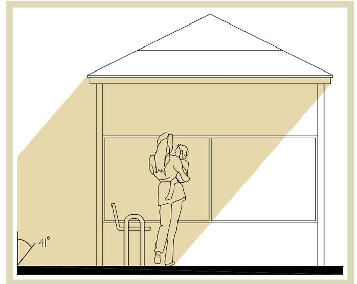
**Fig 1.33** | Approximate angle (41 degree) of the sun during late afternoon peak commuting hours in midsummer in central Florida for a southwest facing bus shelter.
