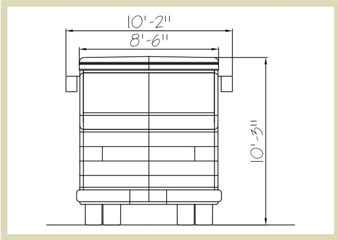
**Fig 2.4** | Front view of a standard 40-foot bus.
