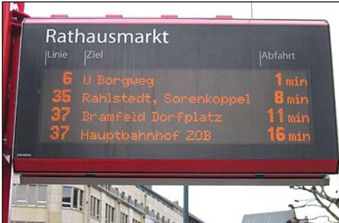
**Fig 1.42** | A digital reader board displaying real-time information about bus arrivals and departures at an inter-modal facility.
