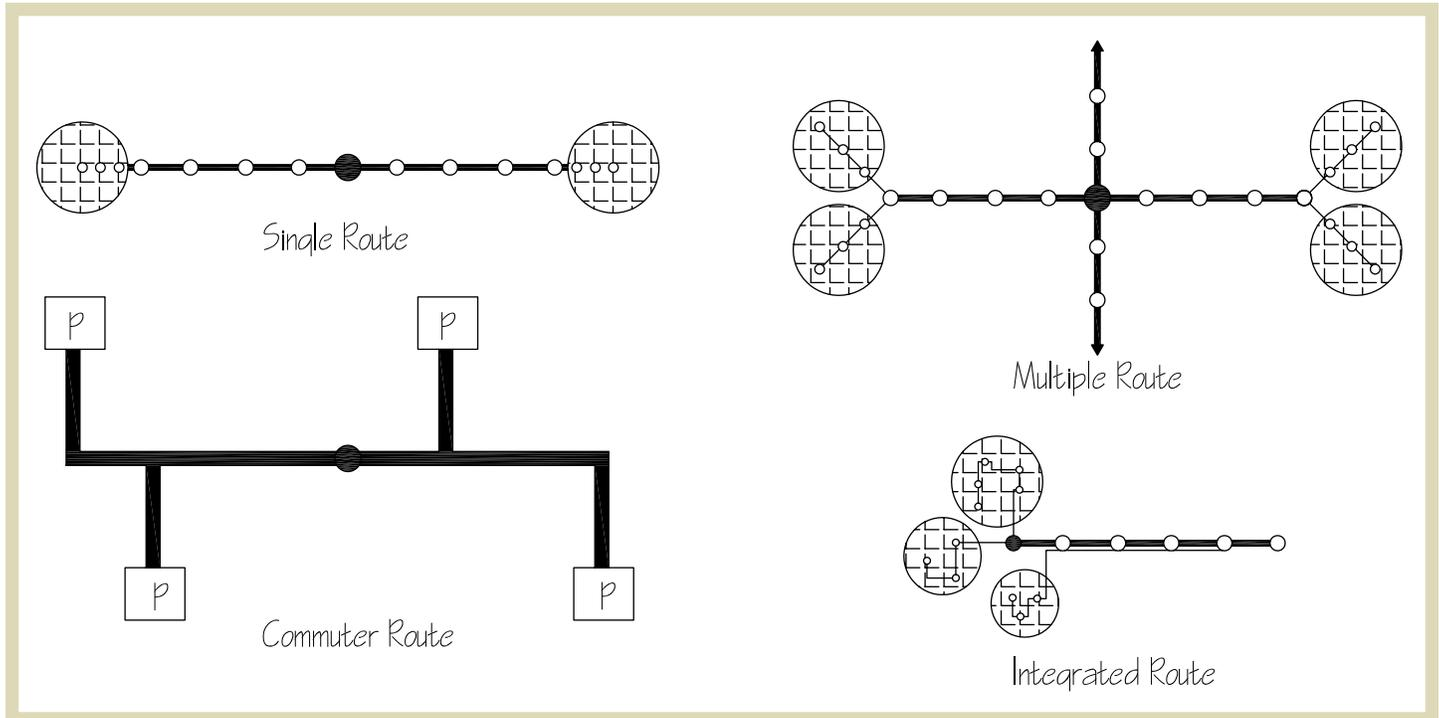
**Figure 3.30** | Typical BRT route alignments.
