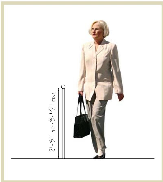
**Fig 1.51** | Correct height dimensions for bus stop leaning rails.
