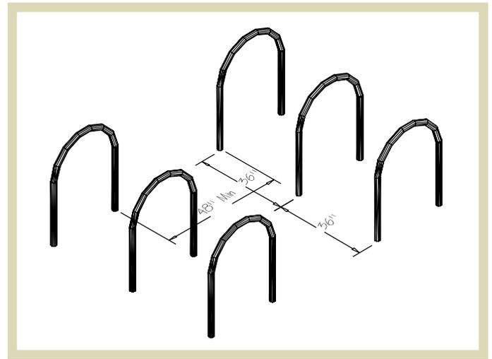
**Fig 1.63** | Spacing for inverted “U” bike racks.
