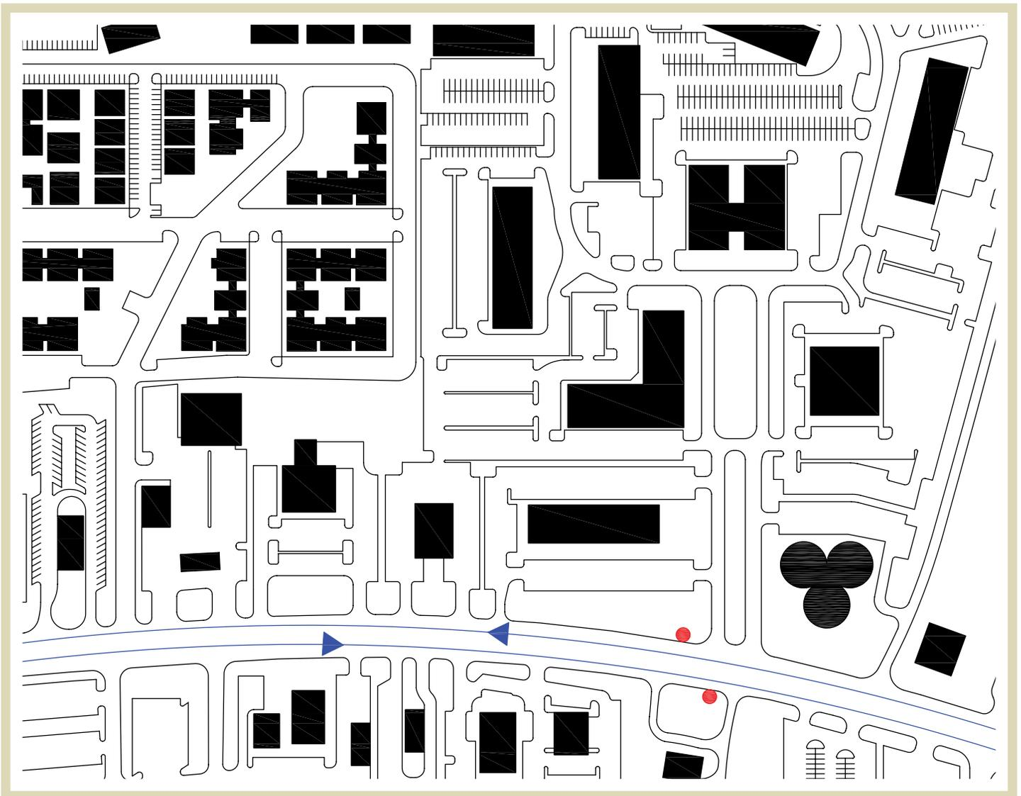
**Figure 4.7** | Mixed use districts along many arterials are often characterized by multiple curb cuts, large block sizes, and poor connectivity between land uses, making them less accessible to both transit riders and pedestrians. Bus stop locations are indicated in red dots in plan.
