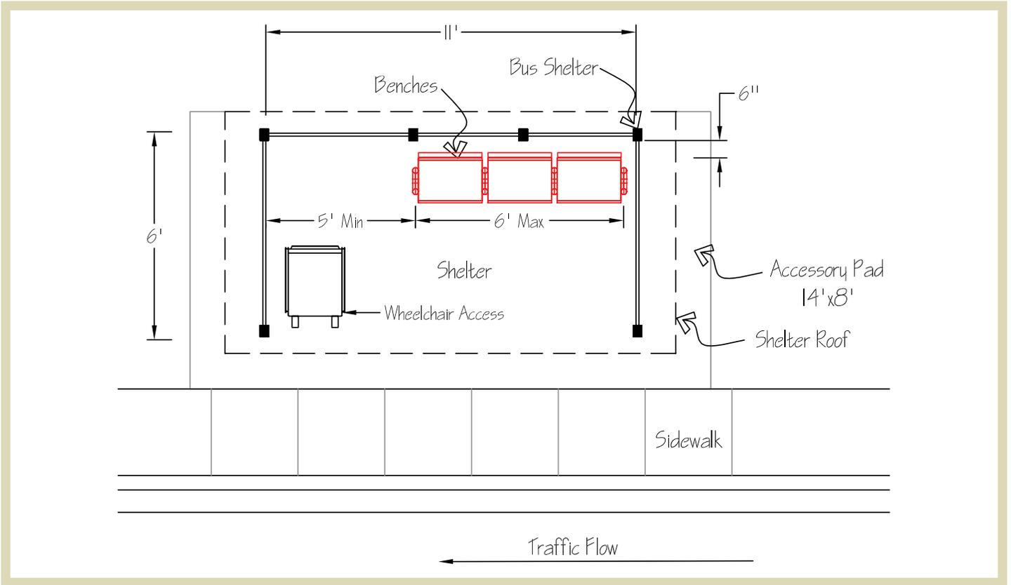
**Figure 1.11** | Locations of bus benches within a bus shelter with opening on one side.
