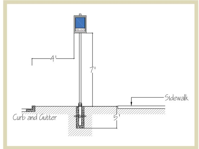
**Figure 1.5** | Dimensions for a bus stop sign placed in a planting strip adjacent to the travel lane.
