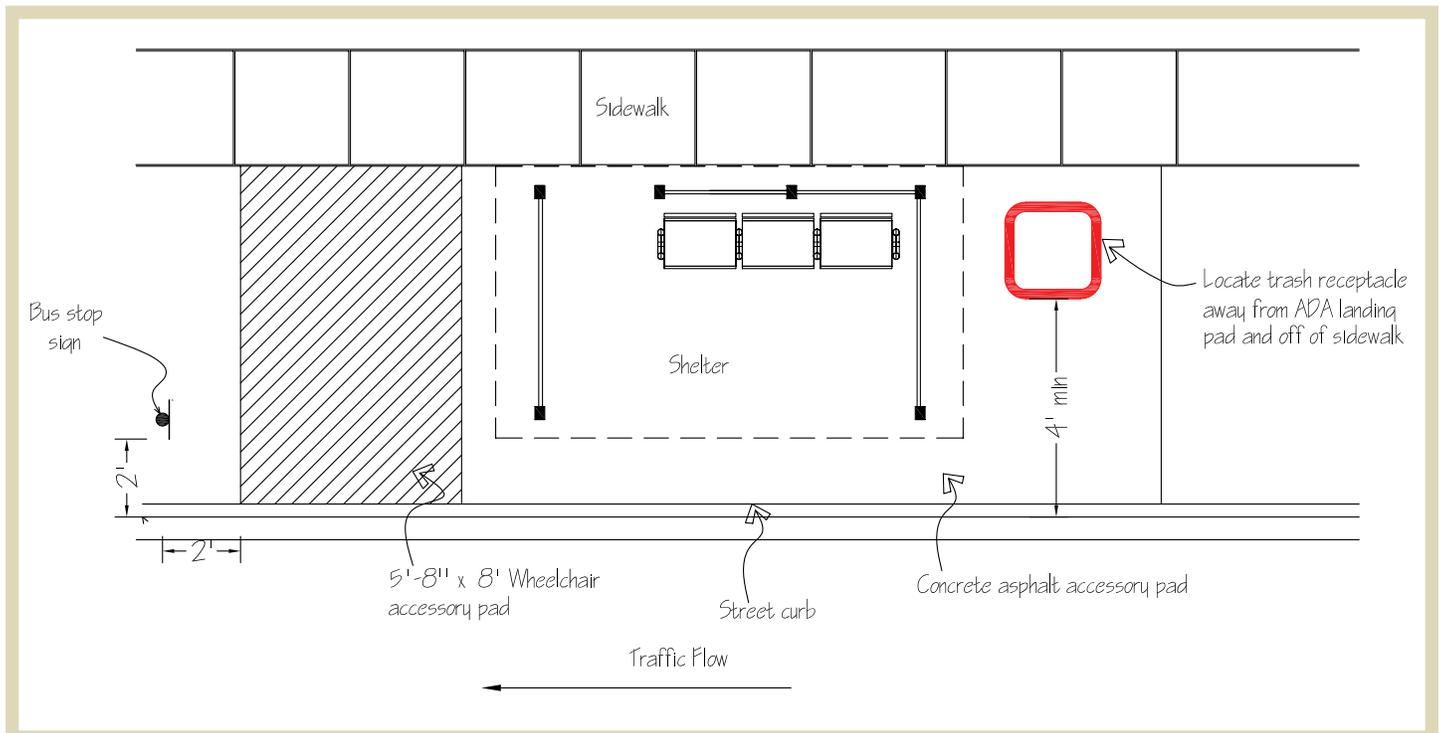
**Fig 1.52** | Correct location of bus stop trash receptacle at a curbside sheltered bus stop.
