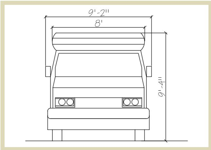
**Fig 2.6** | Front view of a mini bus or para-transit vehicle.
