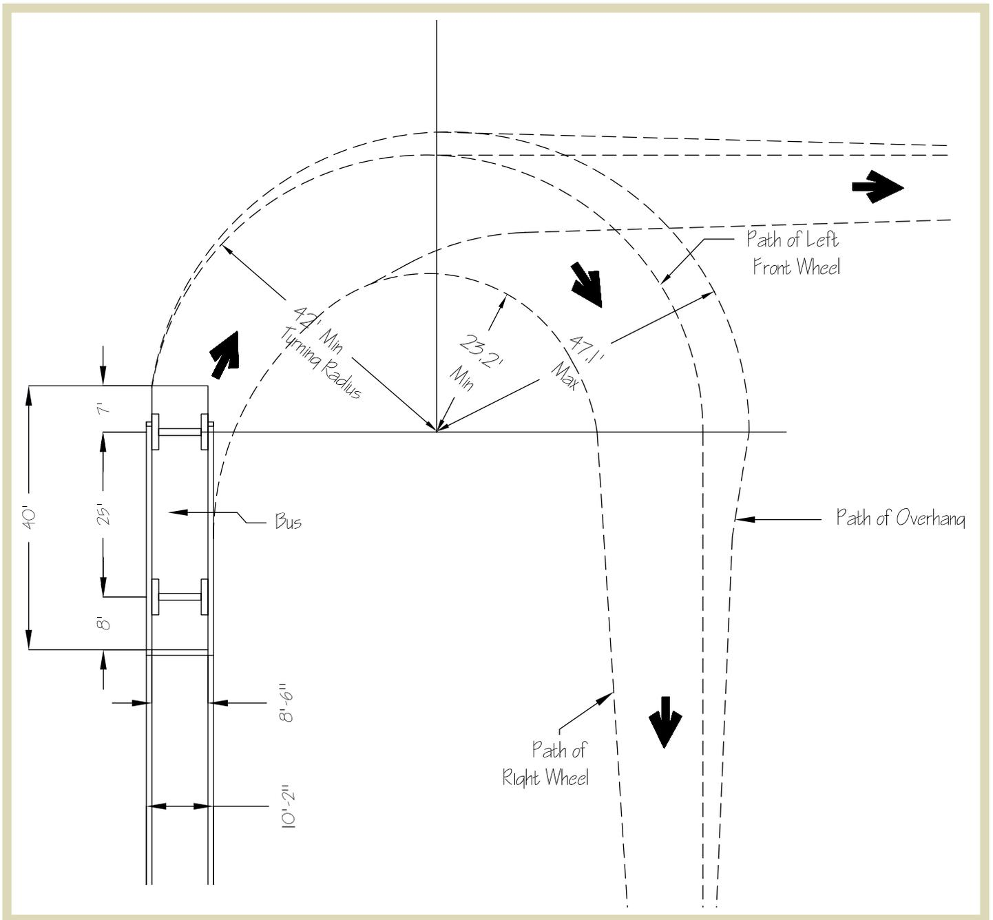
**Figure 2.11** | Template of bus turning movement geometry for a 40-foot bus.
