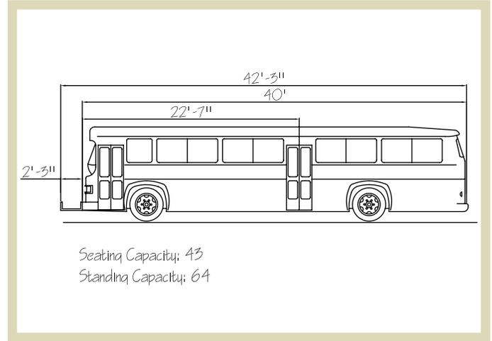
**Fig 2.5** | Side view of a standard 40-foot bus.
