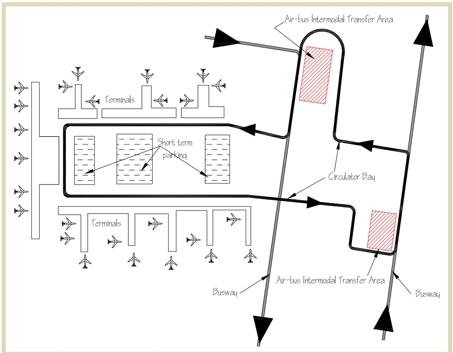
**Figure 3.22** | A typical remote model intermodal center.
