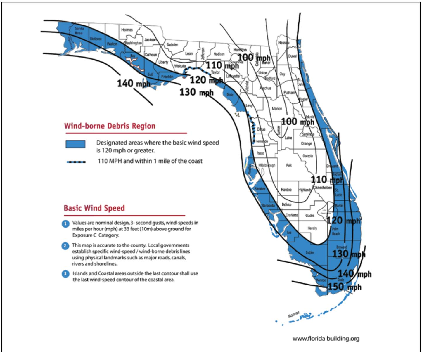
**Fig 1.37** | Design wind speeds for wind loads and wind-borne debris regions used in different areas of Florida, as established by the Florida Building Code.
