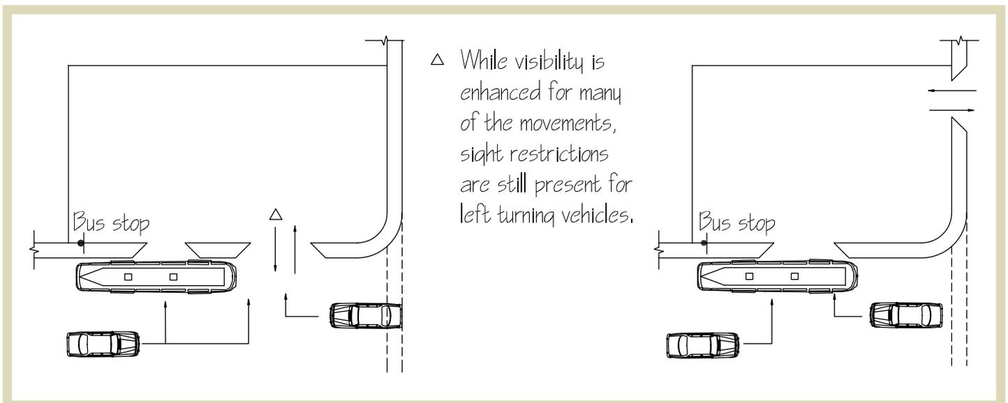
Figure 2.16 | Acceptable bus stop / driveway arrangements.
