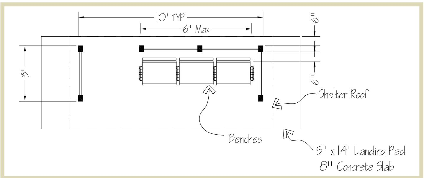
**Fig 1.25** | Typical dimensions of a small bus shelter with seating.
