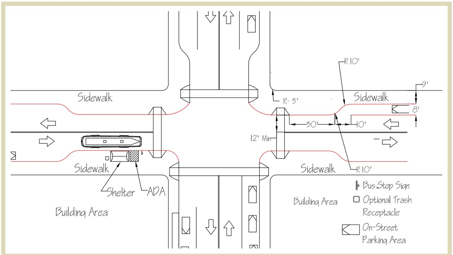
**Figure 2.19** | Dimensions for a bus bulb.
