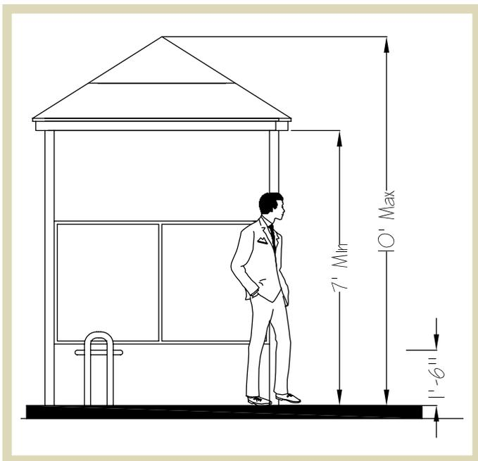
**Fig 1.29** | Cross section of a mid-sized bus shelter, with typical vertical dimensions.
