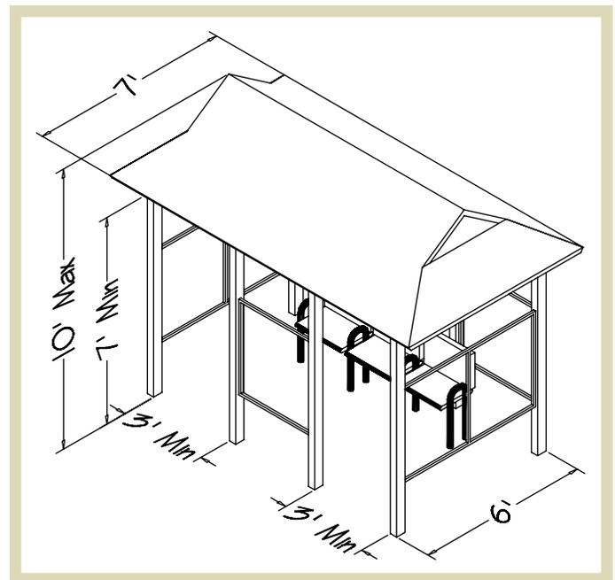
**Fig 1.30** | Mid-sized bus shelter, shown in three dimensions.
