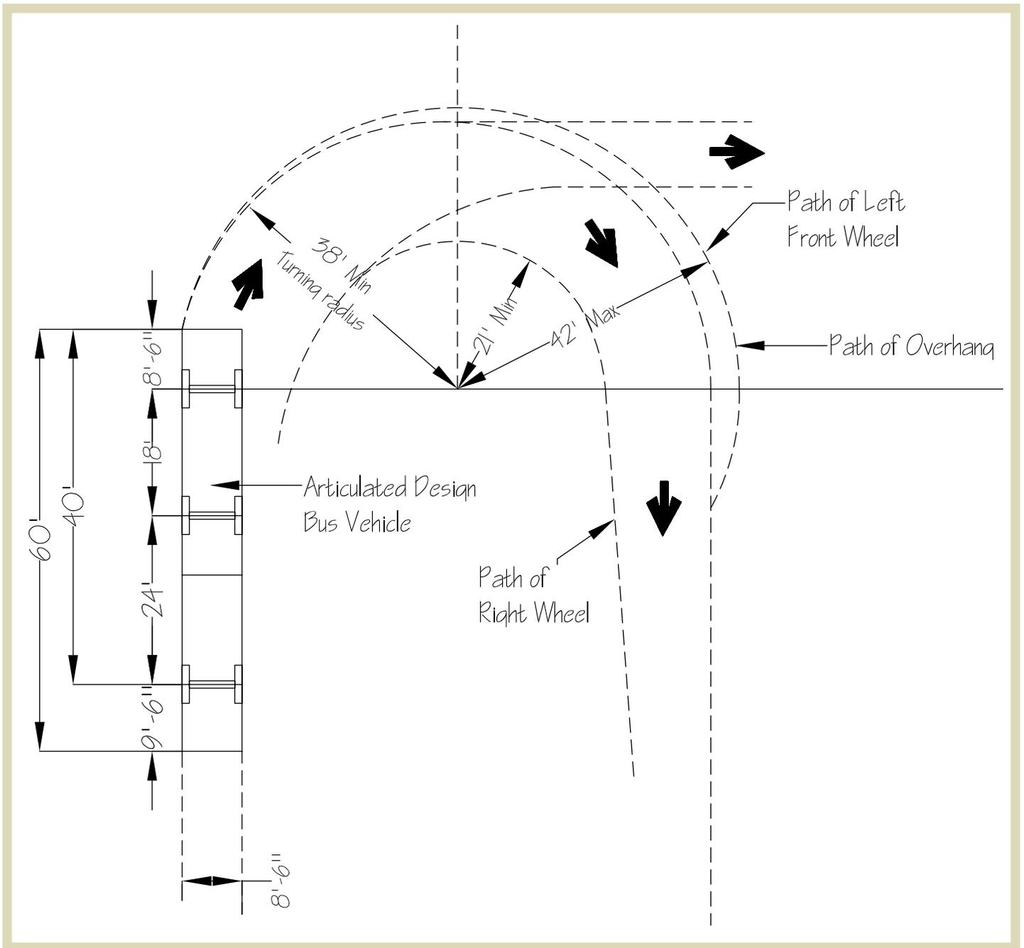
**Figure 2.12** | Template of bus turning movement geometry for a 60-foot bus.
