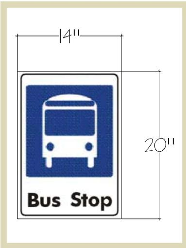
**Figure 1.7** | Typical, but not mandatory, bus stop dimensions for a rectangular bus stop sign.
