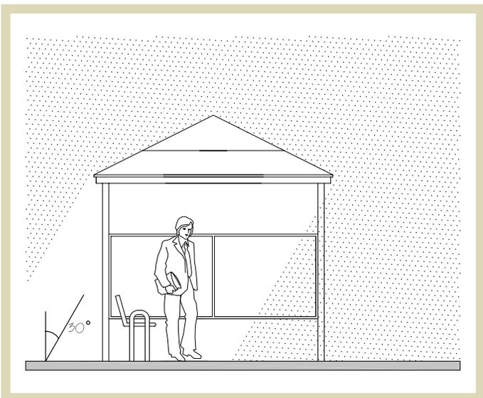
**Fig 1.32** | Typical angle (30 degree) of falling rain in Florida and the related bus shelter canopy required for protection.
