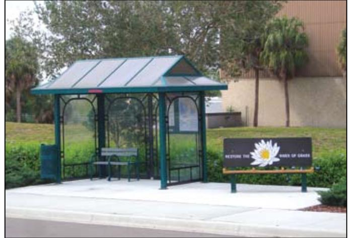
**Figure 1.8** | Correct placement of a bus bench outside of a sheltered bus stop
