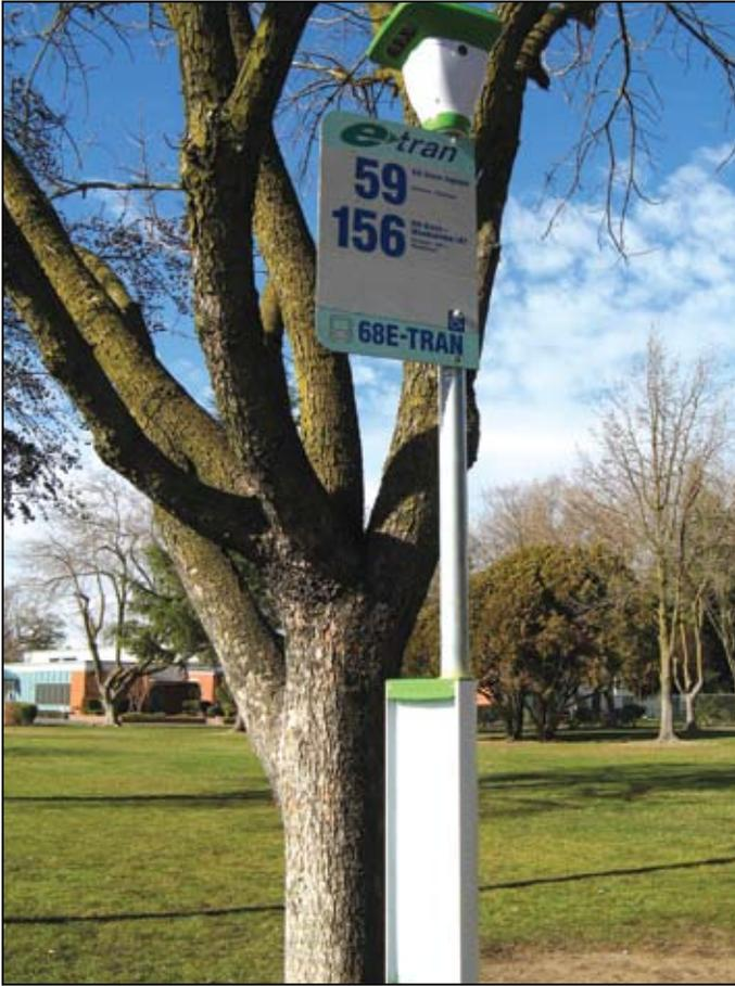
**Figure 1.3** | This solar-powered bus stop signpost provides bus flagging capability and security lighting.
