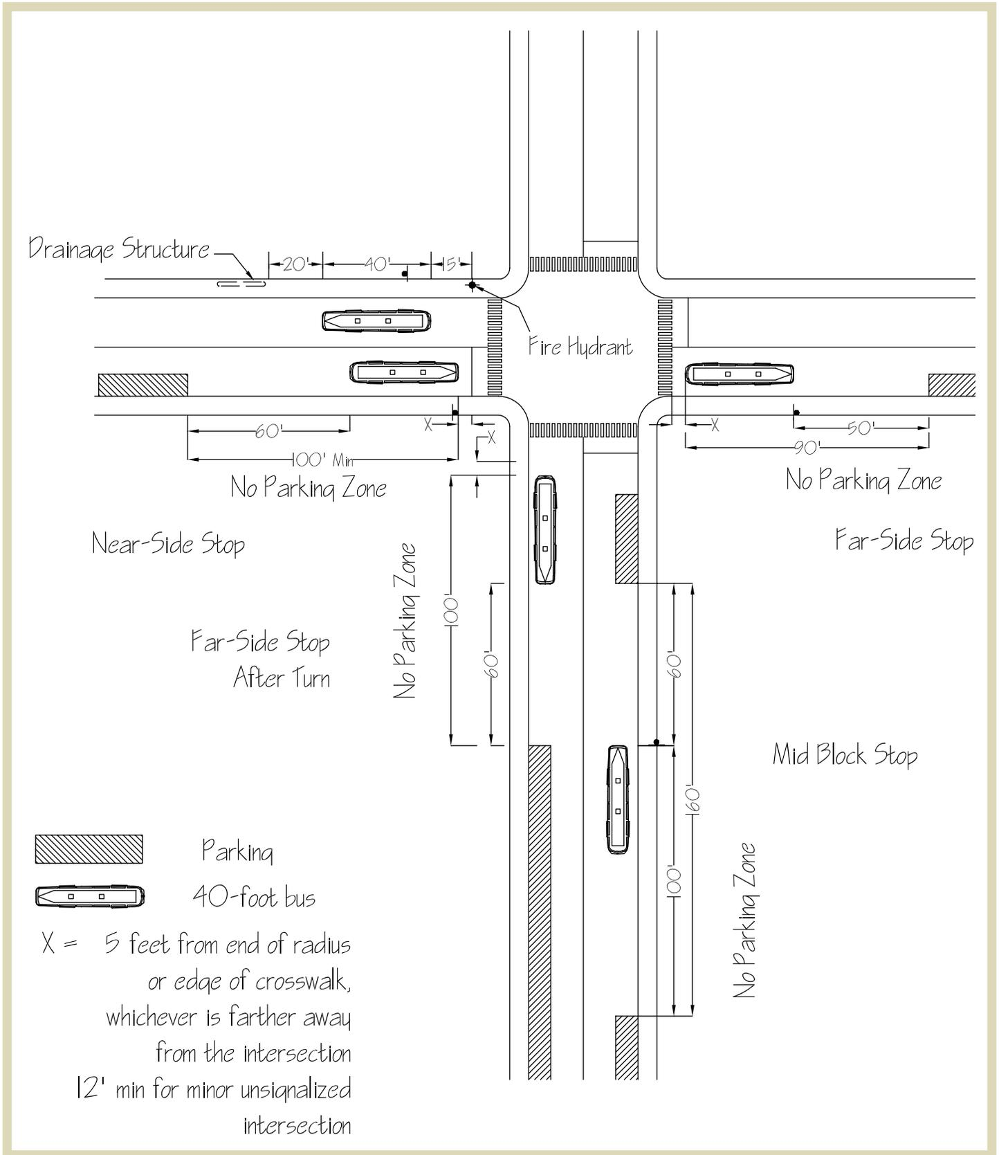
**Figure 2.15** | Dimensions associated with bus stops located at different points with reference to the intersection.
