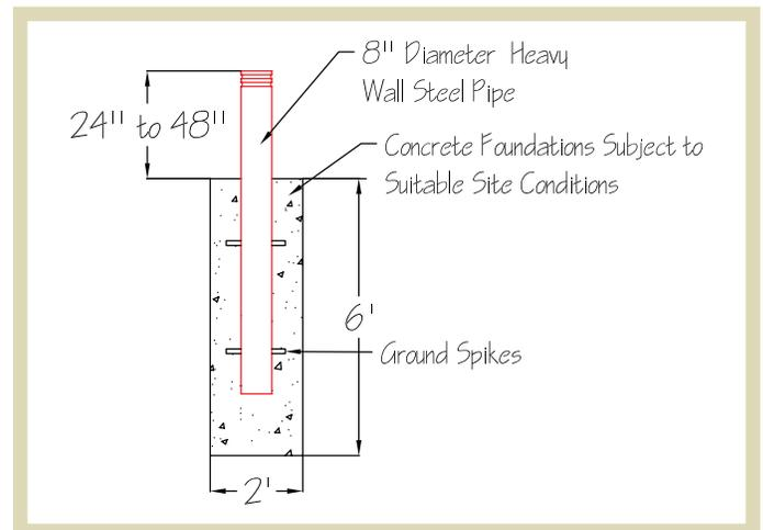
**Fig 1.57** | Detailed section of a typical bollard.
