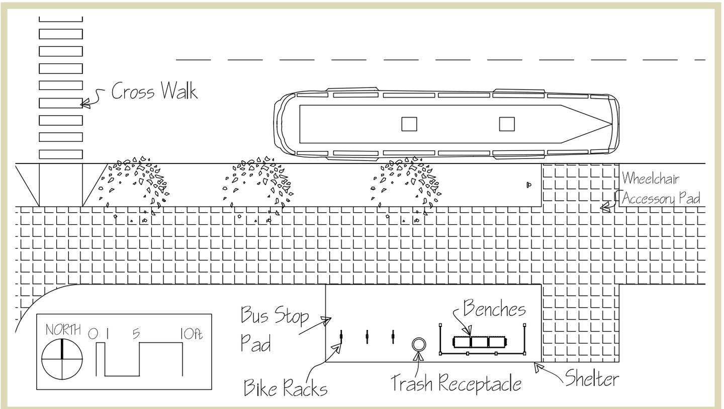
**Figure 3.2** | A detailed plan of an on-line curb-side bus stop.
