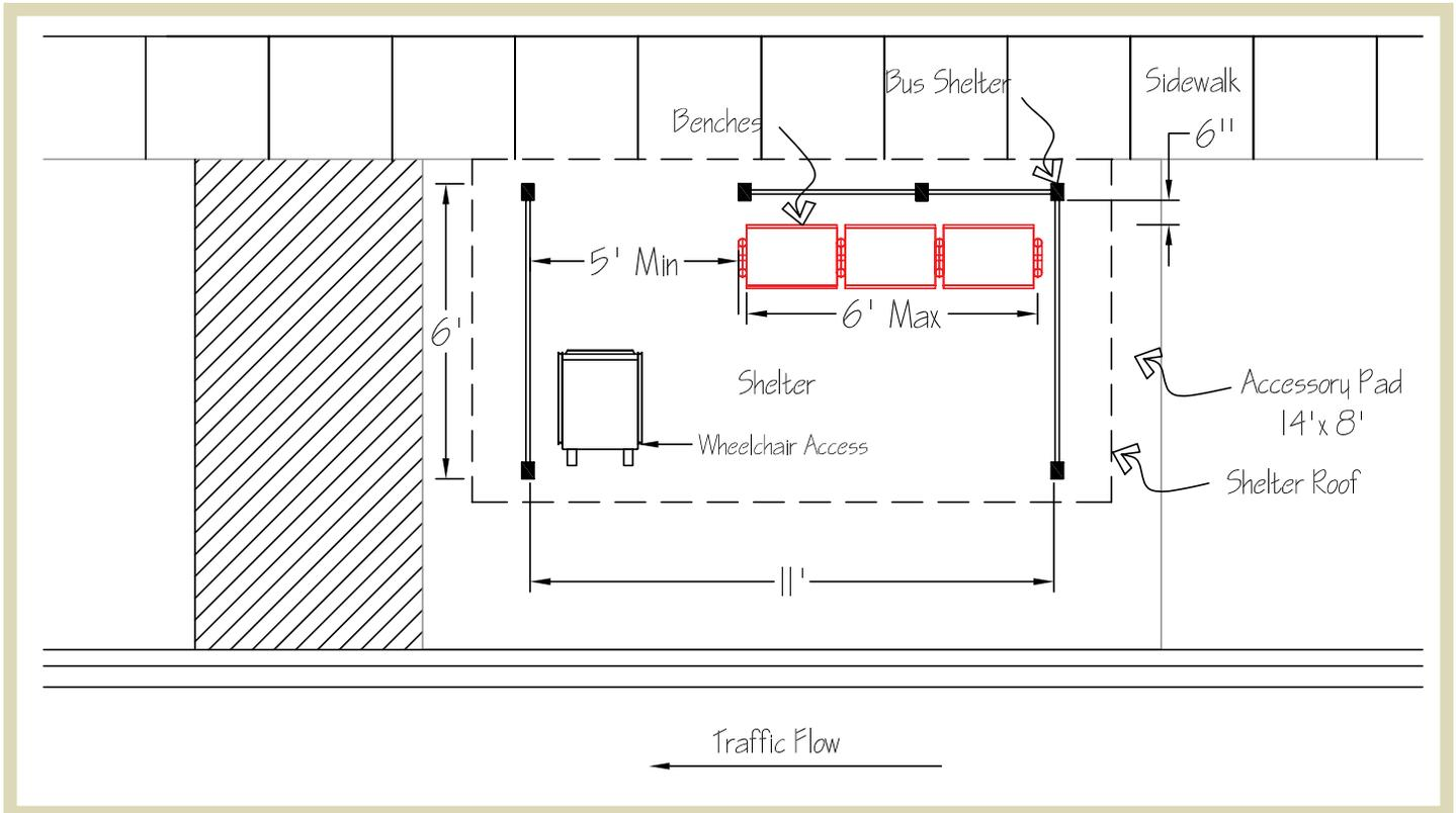
**Figure 1.13** | Locations of bus benches within a bus shelter with different side panel alignment and opening on two sides.
