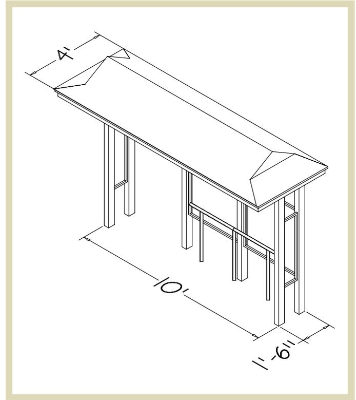
**Fig 1.24** | Small bus shelter with a leaning rail but no seating shown in three dimensions. Plan view of the same bus shelter shown in Figure 1.22.
