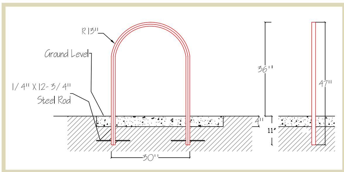
**Fig 1.62** | Critical dimensions for installing an inverted “U” bike rack.
