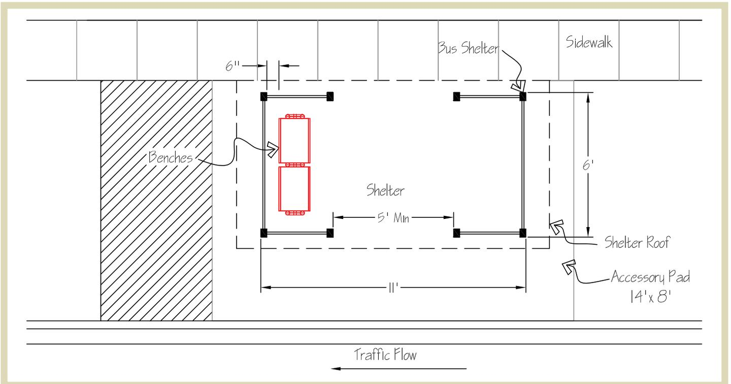
**Figure 1.12** | Locations of bus benches within a bus shelter with opening located centrally on two sides.
