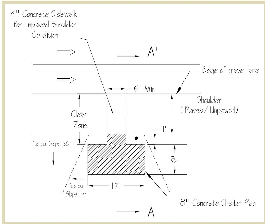
**Figure 1.20 a** | Plan showing landing pad configuration for rural bus stop.
