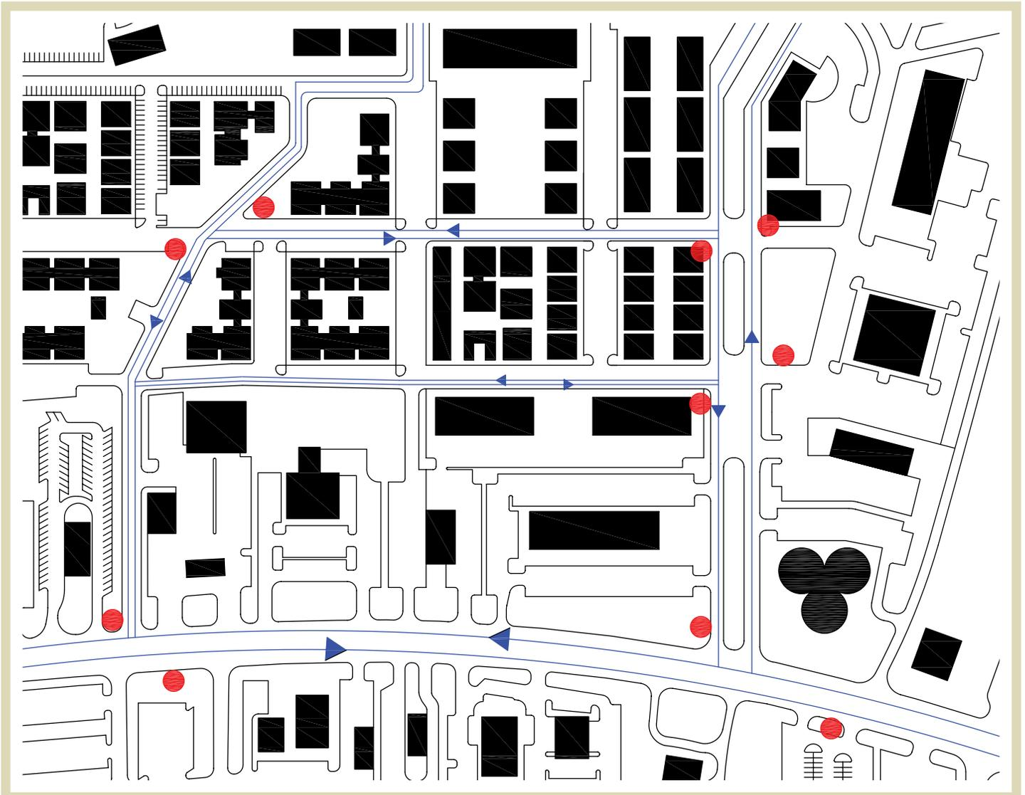
**Figure 4.8** | Mixed use districts along arterials can be made more accessible to transit by reducing the block size and the need for out of direction travel. Bus stops are indicated in red dots in plan.
