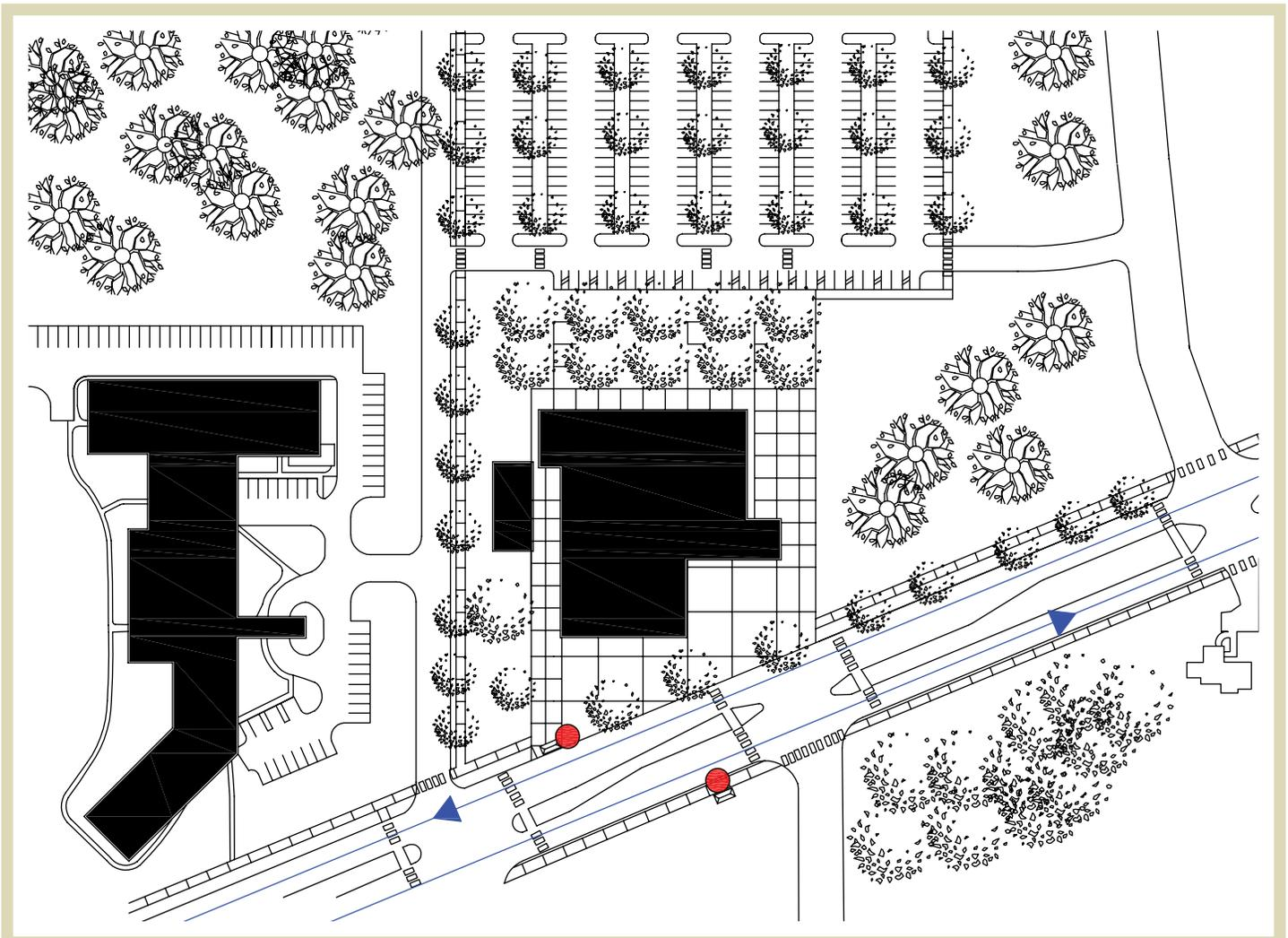
**Figure 4.12** | Simply locating an office building closer to the right of way greatly enhances its accessibility to transit riders and pedestrians. Bus stops are highlighted in red.
