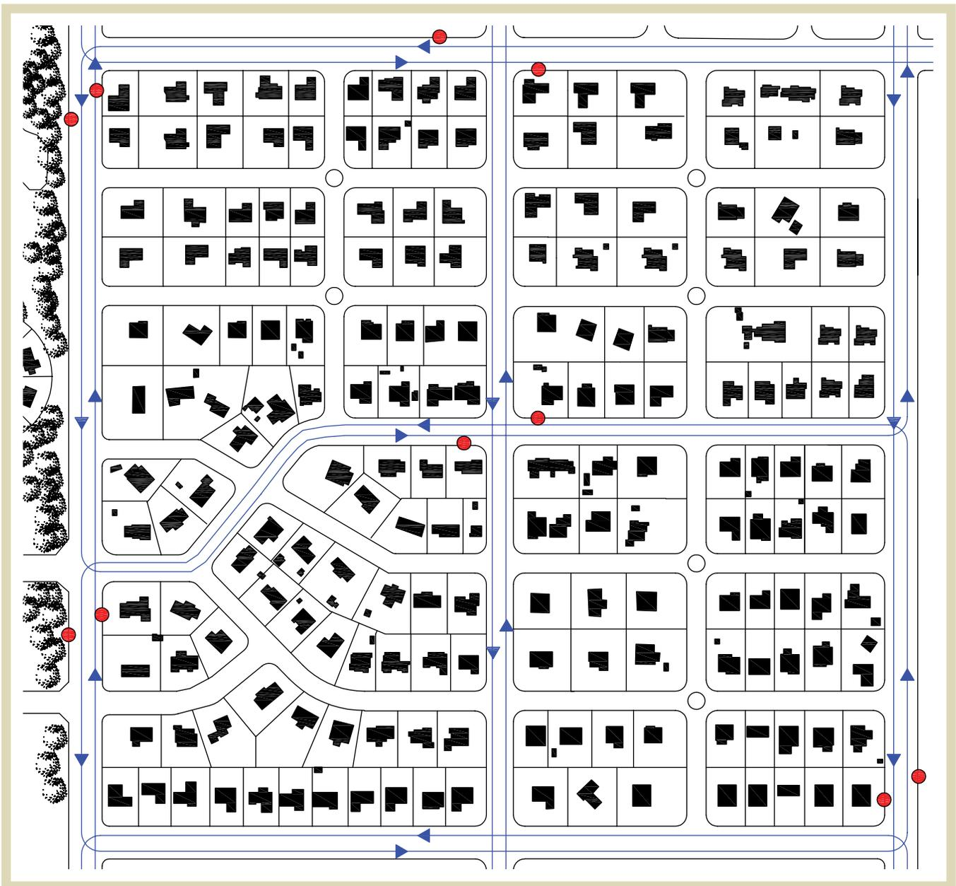
**Figure 4.4** | Transit friendly single family residential development. Bus stops are indicated in red dots in plan.
