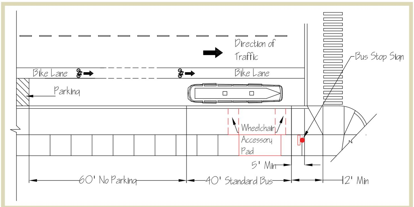
**Figure 2.22** | A typical bike lane-curb side bus stop configuration.
