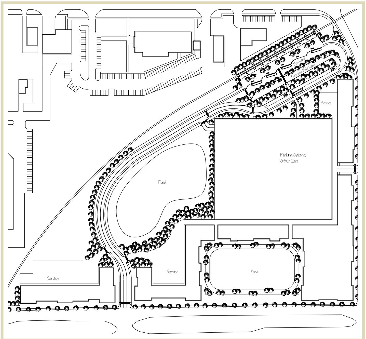
**Figure 3.25** | Plan of a rail bus intermodal transit station in an activity center context.
