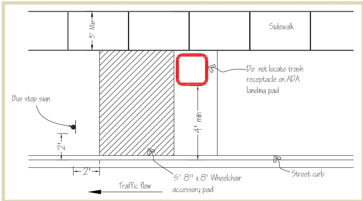
**Fig 1.53** | Correct location of trash stop receptacle at a curbside bus stop without shelter.
