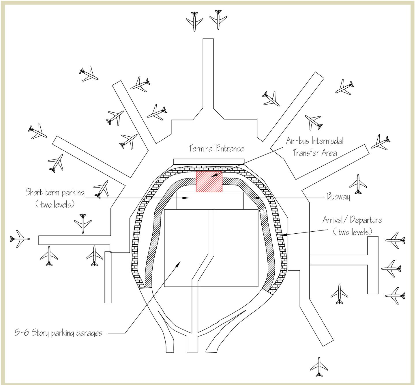
**Figure 3.21** | A typical proximate model intermodal center.
