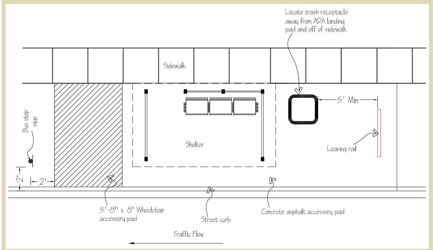
**Fig 1.49** | Correct location of a leaning rail located outside a bus stop shelter.
