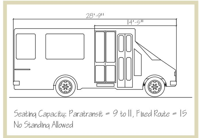
**Fig 2.7** | Side view of a mini bus or para-transit vehicle.
