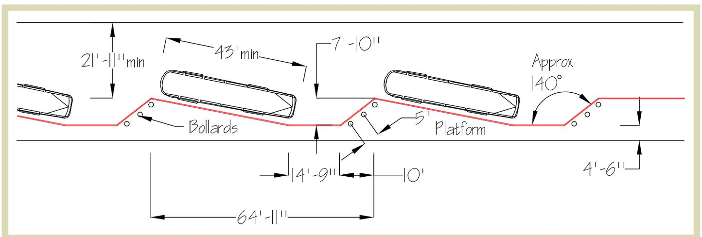
**Figure 2.20** | Dimensions for an off-street half-sawtooth bus bay for a 40-foot bus equipped with a bike rack.
