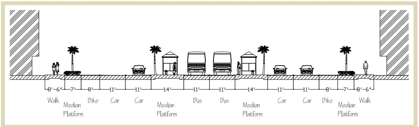
**Figure 3.9** | Cross-section of the right of way for a transit mall.
