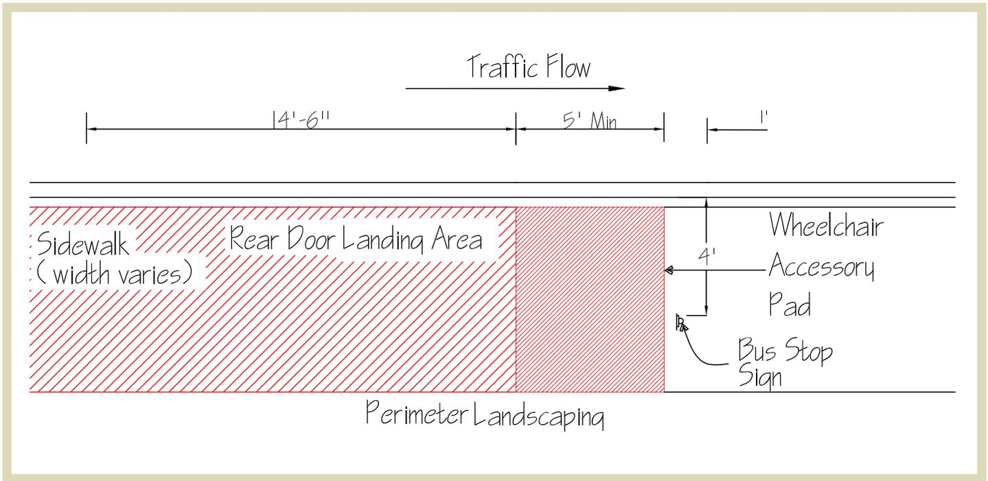
**Figure 1.19** | Landing pad configuration when the sidewalk is directly adjacent to the curb.
