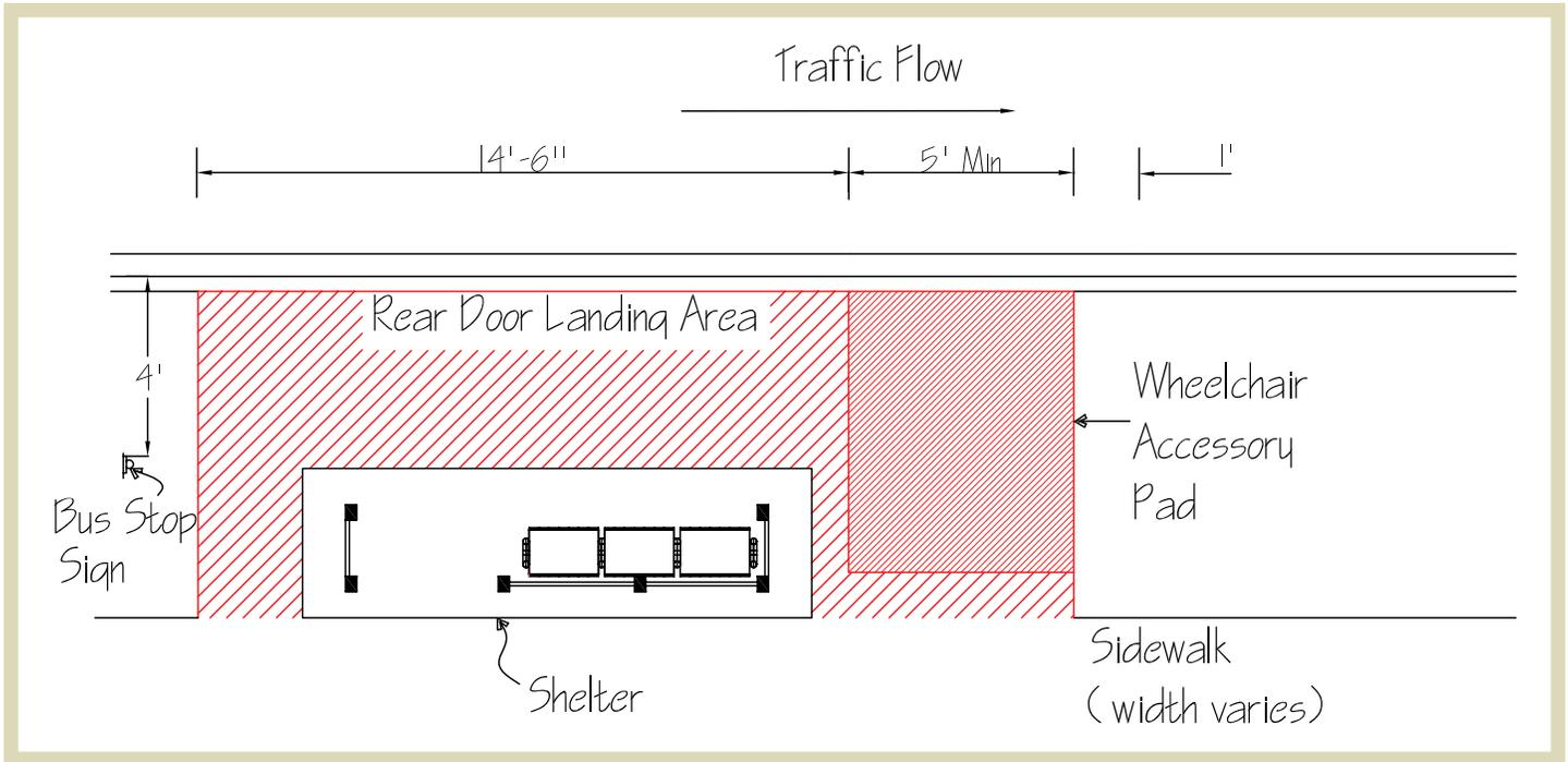
**Figure 1.16** | Bus stop pad with shelter.
