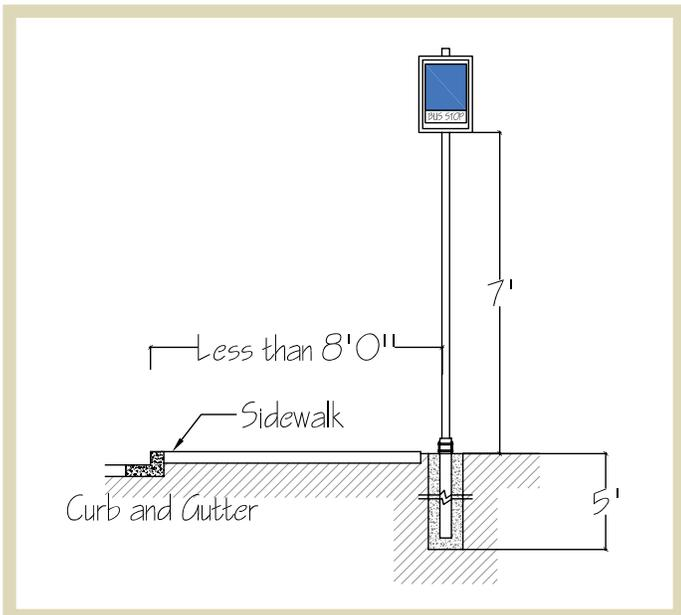
**Figure 1.4** | Dimensions for a bus stop sign placed on the far side of a sidewalk adjacent to the travel lane.
