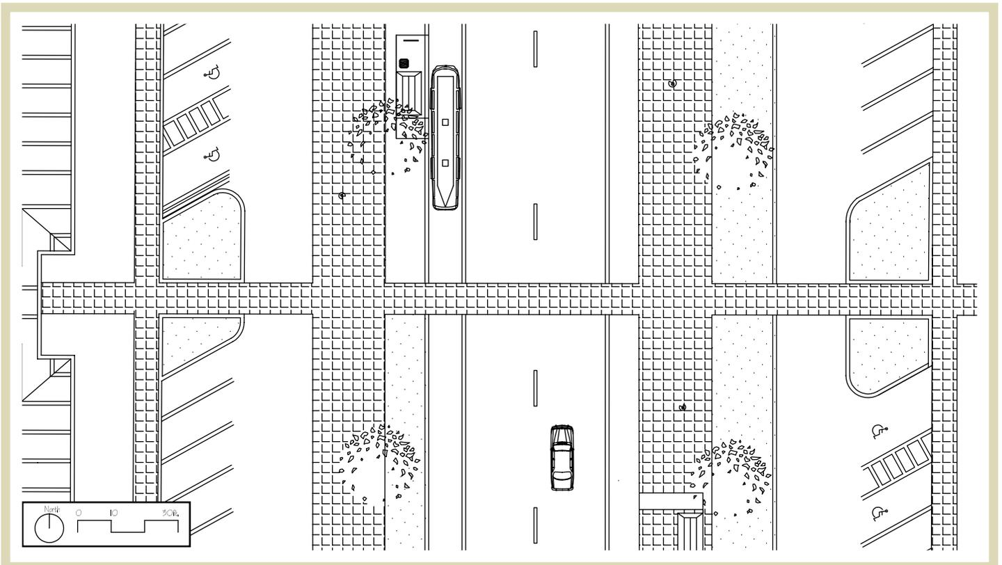
**Figure 3.6** | A detailed plan of a primary bus stop.
