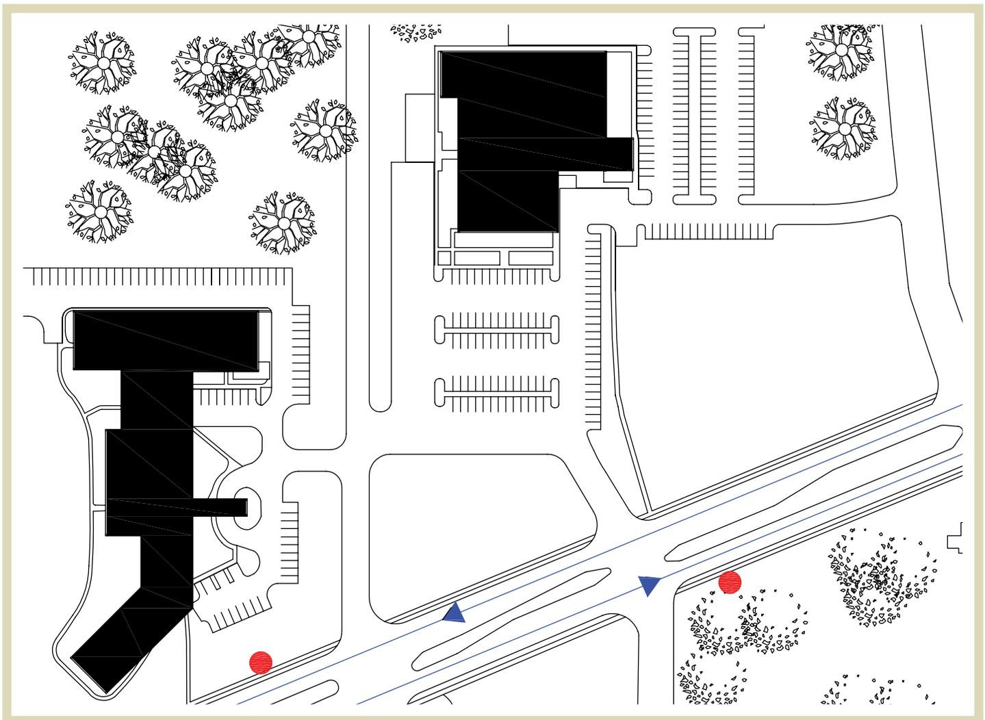
**Figure 4.11** | Many office buildings are set back from the right of way, causing increased trip length and reduced accessibility for transit riders and pedestrians. Bus stops are indicated in red dots in plan.
