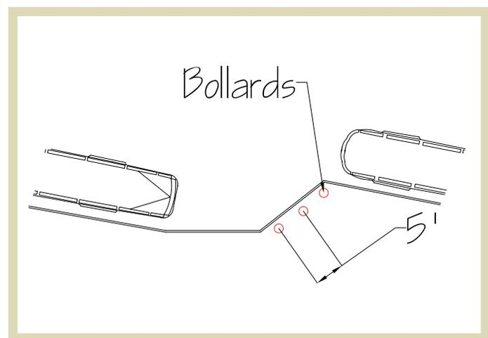
**Fig 1.58** | Plan showing bollards in an off-street half saw-tooth bus bay.
