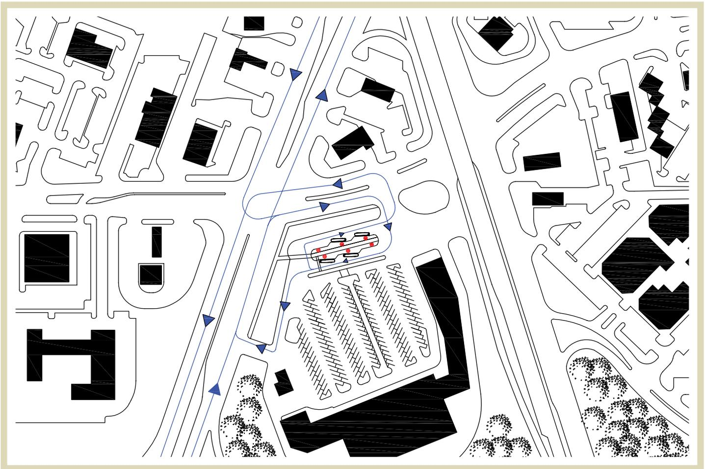
**Figure 4.9** | Many shopping centers are separated from the street by large parking lots, causing transit riders and pedestrians to negotiate many conflicts with automobile traffic. Bus stops are indicated in red dots in plan.
