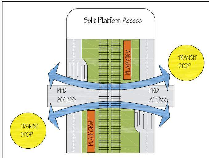
**Figure 3.29** | Diagram of a split platform station.
