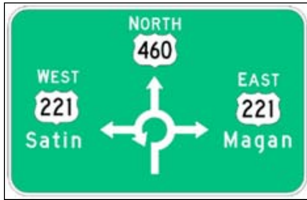
FIGURE 3 Diagrammatic roundabout guide sign.
