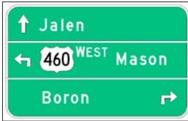
FIGURE 2 Maryland roundabout guide sign.
