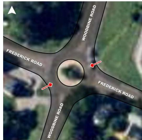
Taking the above into consideration, this lighting arrangement is not practical for most applications. However, in a rural environment with no pedestrians and where funding for installation and maintenance of lighting equipment is limited, this would be a useful approach. However, higher levels of lighting would be far better if at all possible and should be installed whenever possible.
