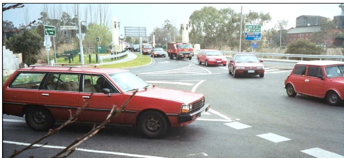
Figure 2 - An example of dominant entry flow at a modern roundabout: Grange Rd, St Georges Rd and Alexandra Avenue in Toorak, Melbourne, Australia (photo modified for driving on the right-hand side of the road)
