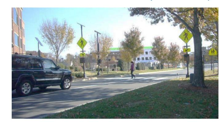
These devices provide an irregular, LED flashing indication when activated.
