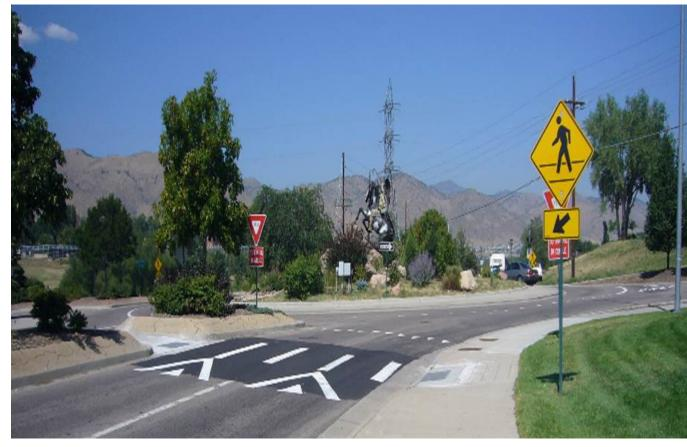
A crosswalk at the elevation of the sidewalk rather than the elevation of the roadway.
