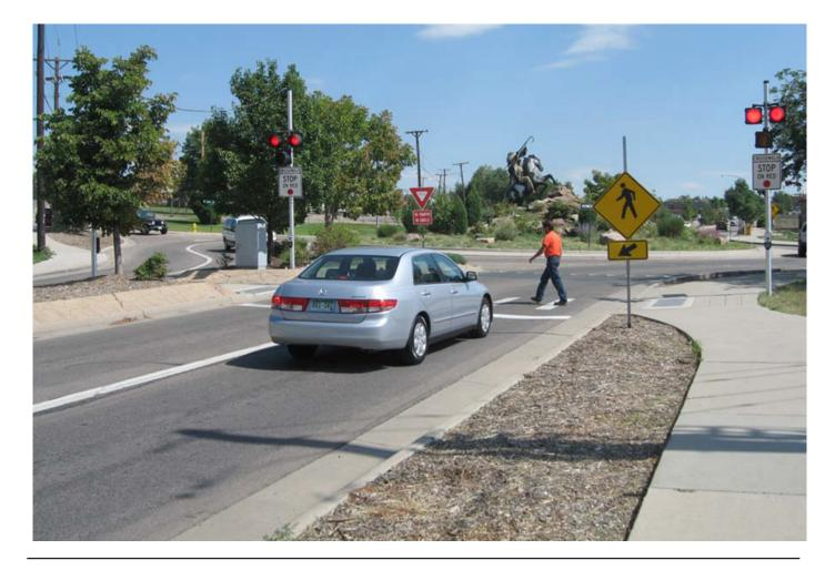
Formerly known as HAWK signals, these devices provide a series of indications to drivers when activated, including a steady red indication.
