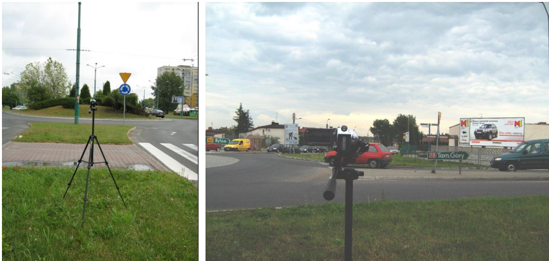
Figure 1 - Traffic surveys using digital video cameras
