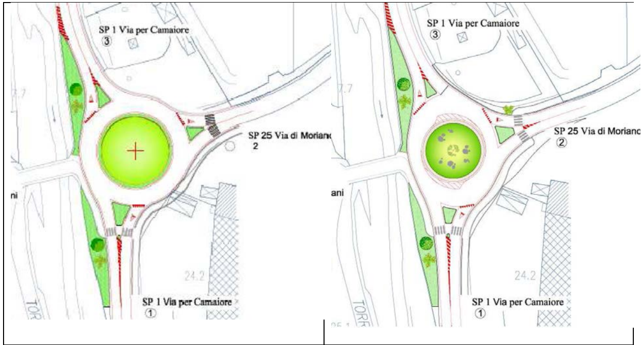
Figure 4. Test intersection layout with full centerline offset, or tangent: conventional roundabout (left) and two-geometry roundabout (right).
