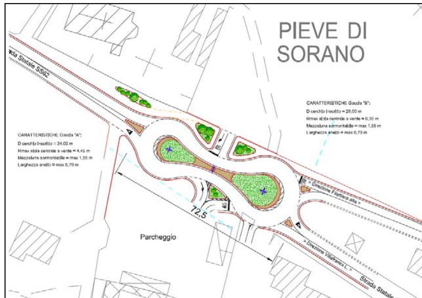
Figure 2. A compact double-teardrop layout designed for a constrained intersection in Filattiera (Italy).
