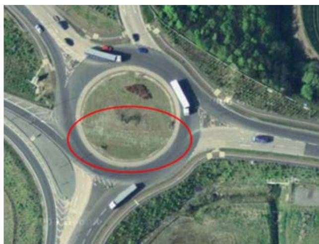
Figure 16. An example from the UK of a turf-stabilized center island (photo by David Collett, Collett & Sons Ltd.)
