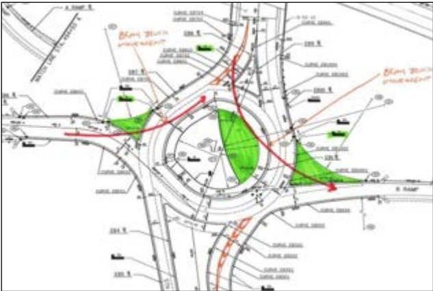
Figure 13. Slide showing schematic of possible OSOW turning movements through a roundabout (Slide from Mark Lenters, Ourston Roundabout Engineering)
