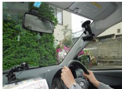
FIGURE 2 The equipped experimental vehicle and the setting of in-vehicle video cameras
