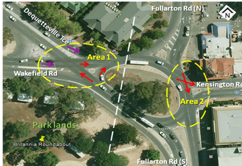
Figure 2. Two major crash areas of the Britannia roundabout
