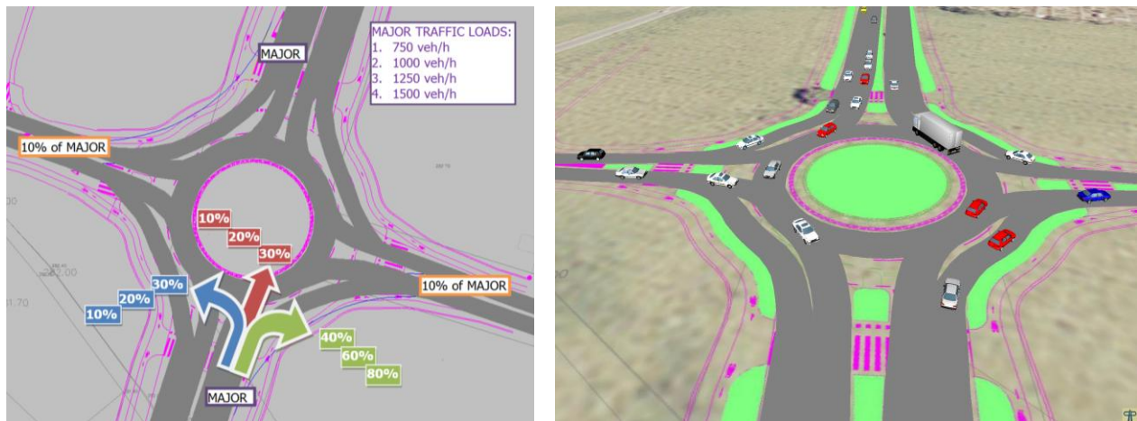
Figure 9 - The mathematical model and 3D simulation of "depressed" roundabout with PTV VISSIM 5.20
