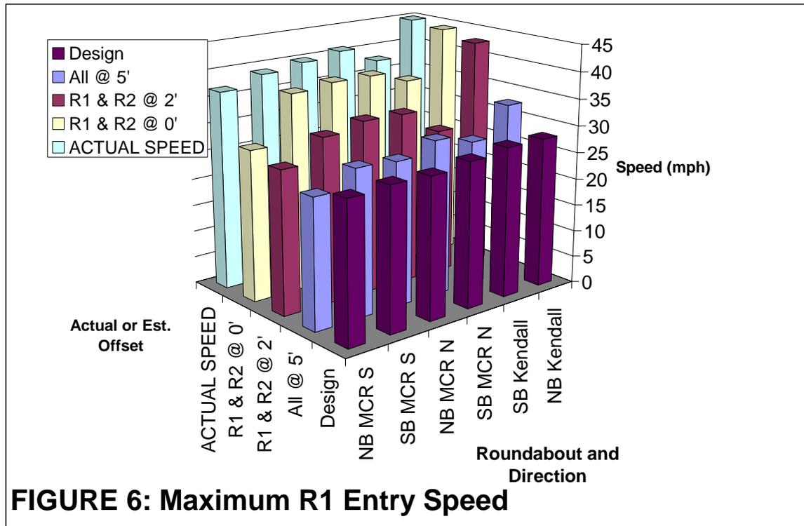
As discussed above, the professional estimate and City verification, using standard fastest path procedures with a 5-foot offset, appear to coordinate well. This does not hold true for NB Kendall Parkway where the designer predicted a
