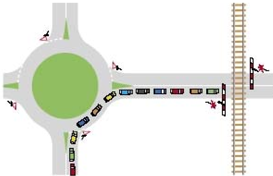
Figure 3 – Railroad Crossing Queue Backing Into Roundabout
