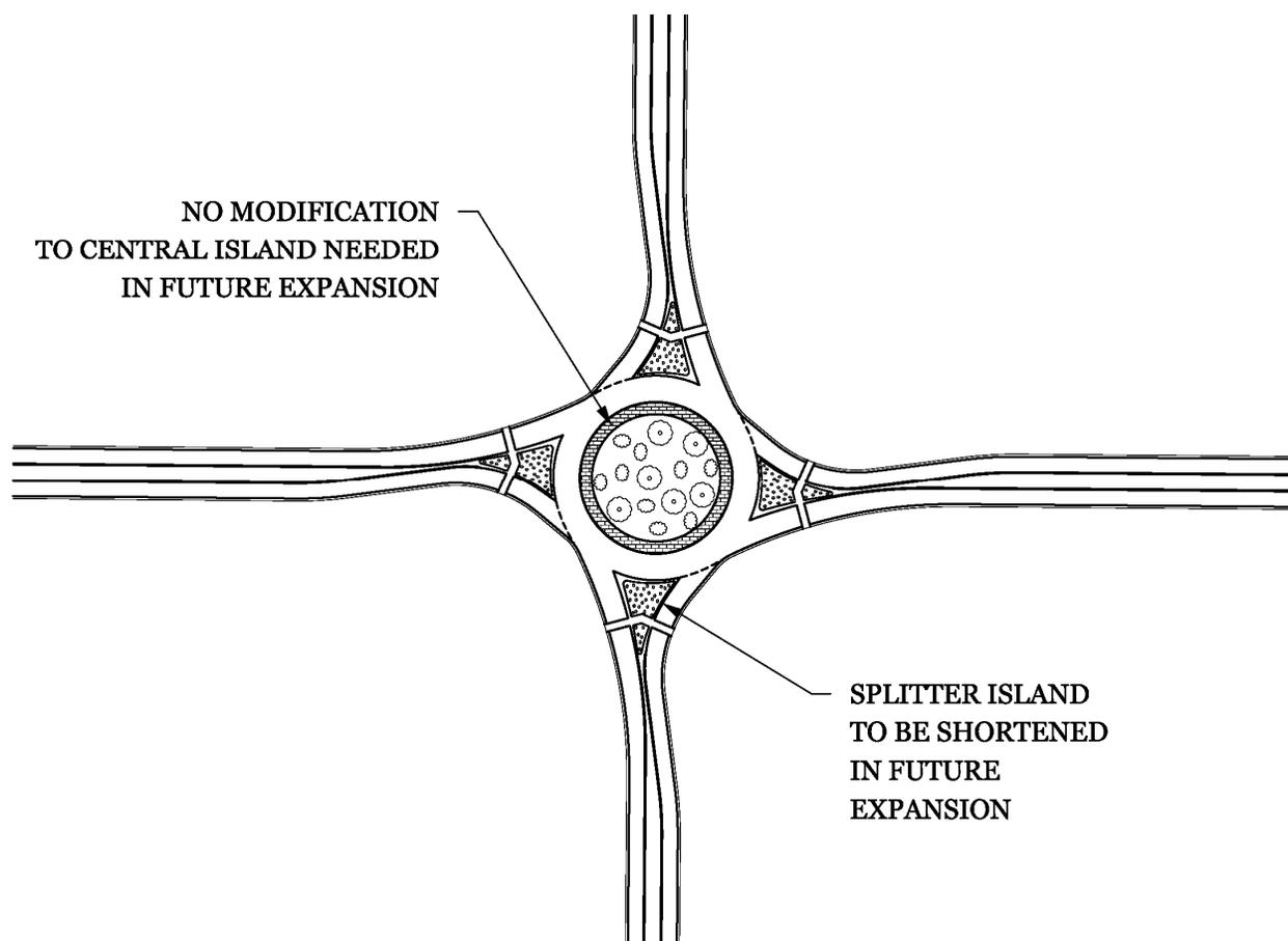
**FIGURE 3** Example of initial inside build with future widening outward.
