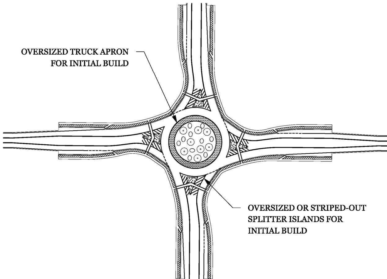
**FIGURE 2** Example of initial outside build with future inward widening.
