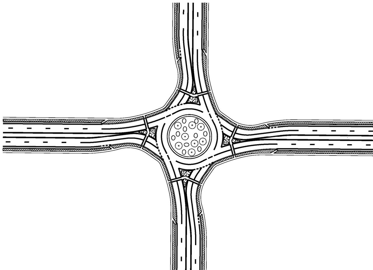
**FIGURE 1** Example of dual-lane roundabout layout.
