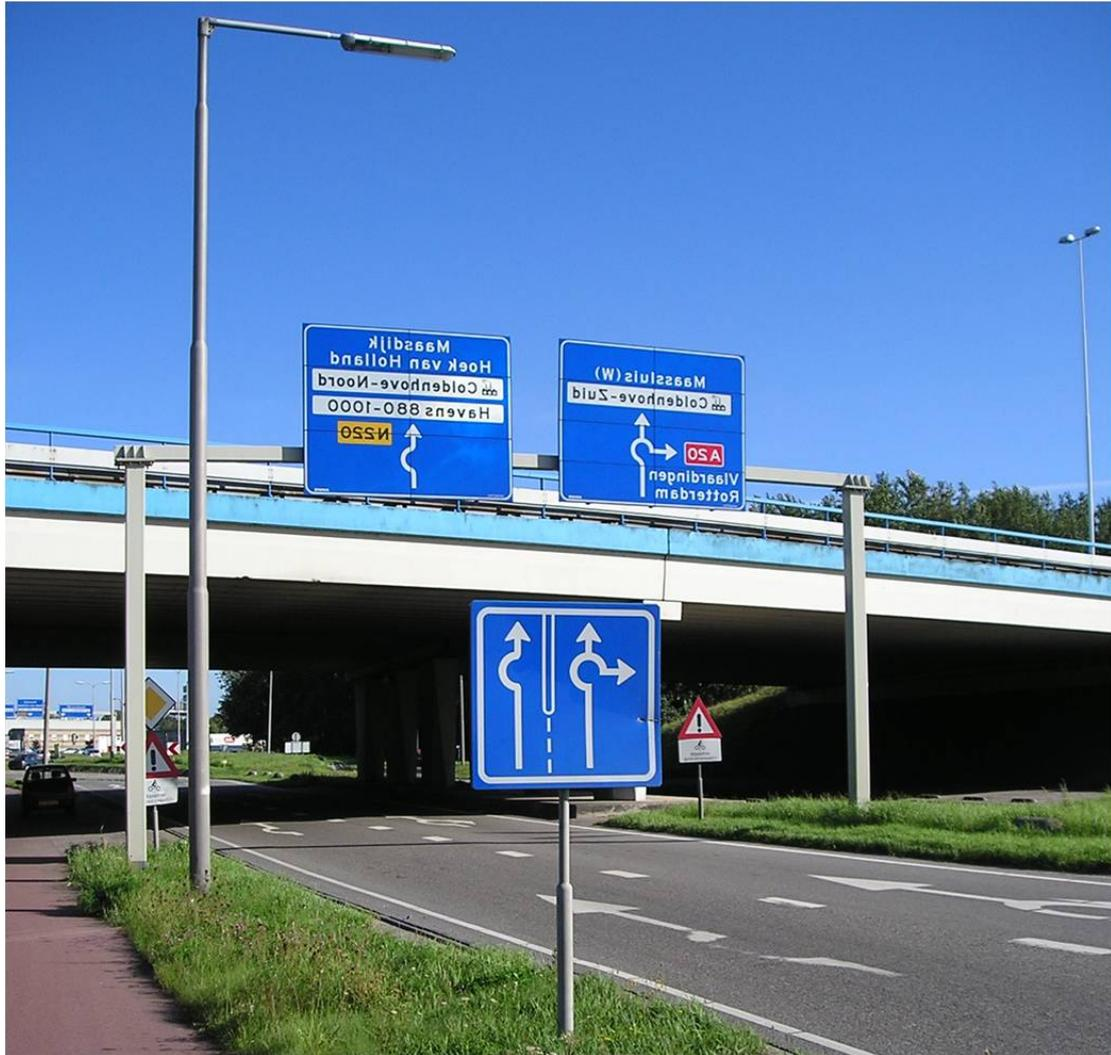
**FIGURE 11** Road Signs to assist entry lanes at roundabouts in The Netherlands
